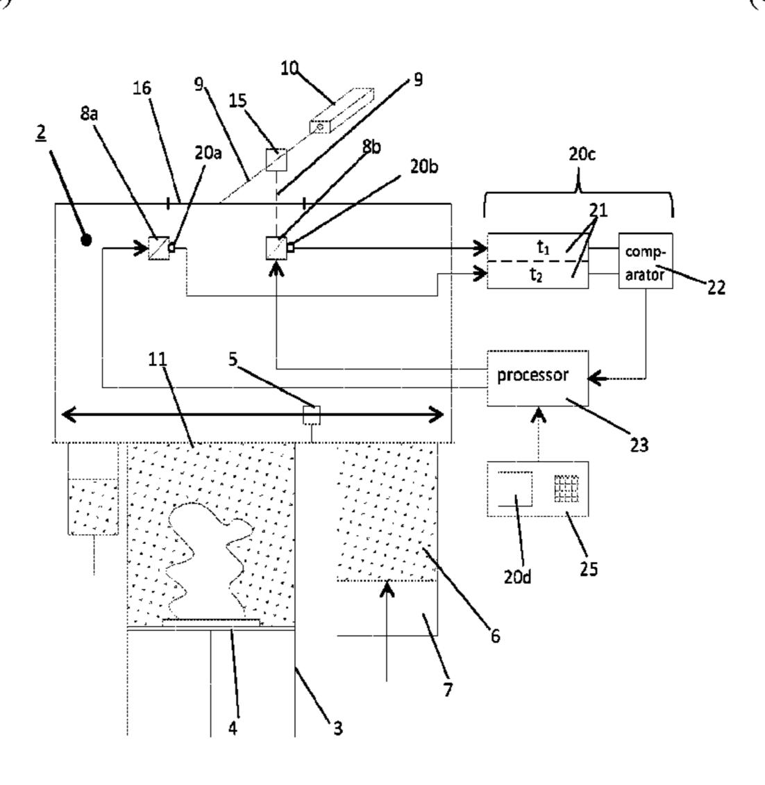
is indicative of a time required for the second scanner to irradiate the second region with respect to at least one of the plurality of sequential layers of construction material. The first irradiation time and the second irradiation time may be at least approximately the same.
