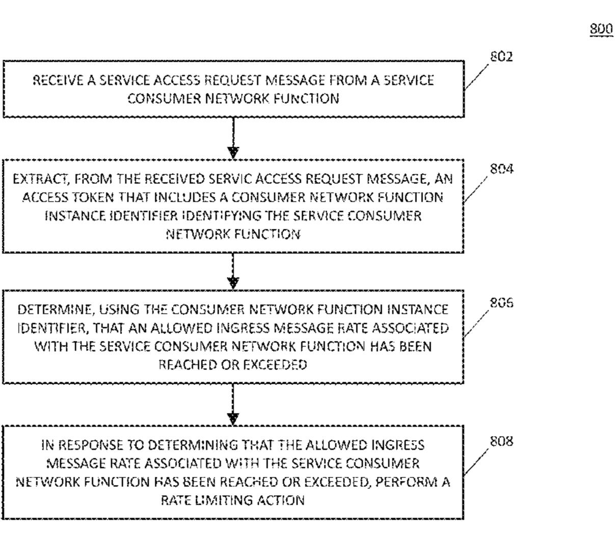
function has been reached or exceeded and in response to determining that the allowed ingress message rate associated with the service consumer network function has been reached or exceeded, performing a message rate limiting action.
