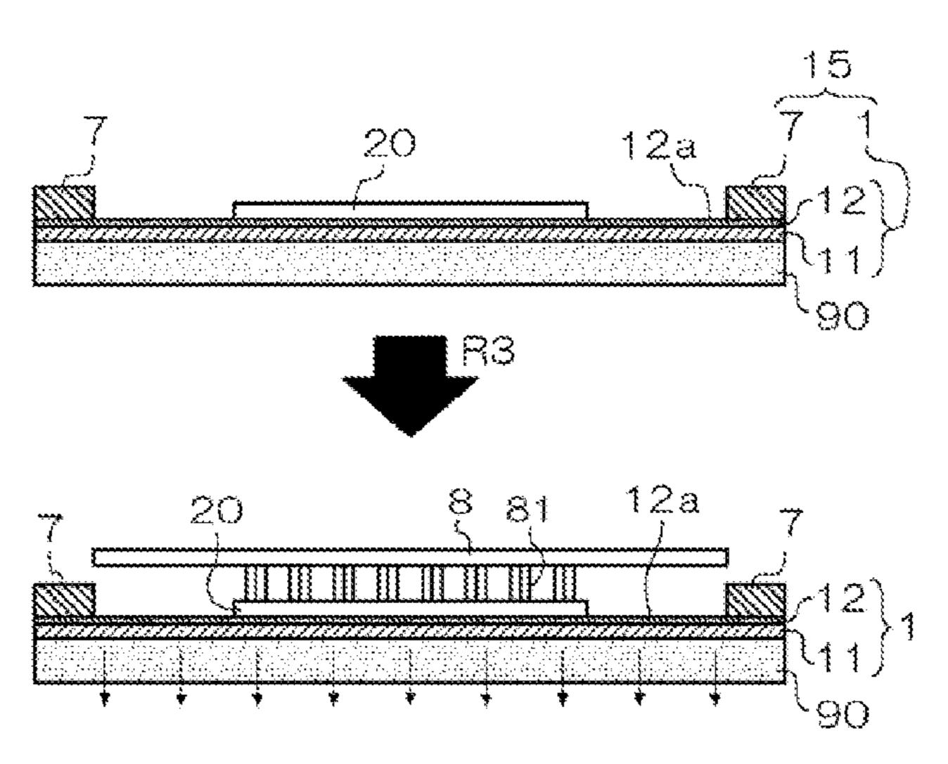
the film for component manufacture includes a segmenting step, a pickup step, and an evaluation step prior to the pickup step.
