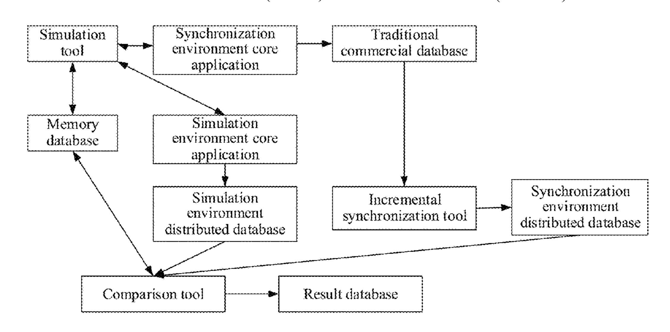
between the message values. The result database is configured to store comparison result data generated by the comparison tool.
