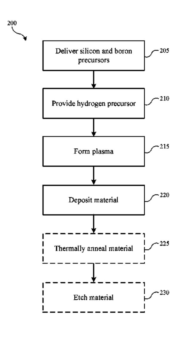
include depositing a silicon-and-boron material on a substrate disposed within the processing region of the semiconductor processing chamber.
