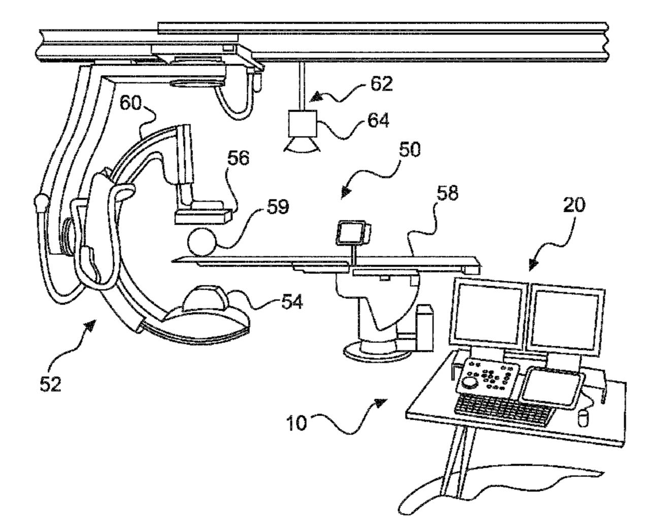
tions for movement of the 3D motion-model. The processing unit is configured to adapt the 3D motion-model according to the movement instructions. The processing unit is also configured to generate a virtual X-ray projection of a region of interest based on the spatial arrangement of the 3D motion-model in relation to the 3D model of the subject. Further, the output unit is configured to provide image data of the virtual X-ray projection.
