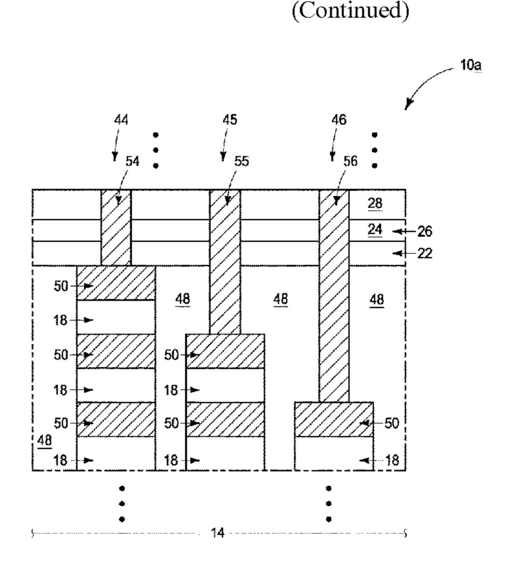
memory array region. A staircase region is proximate the memory array region. The staircase region has electrical contacts in one-to-one correspondence with the conductive levels. A layer is over the memory array region and over the staircase region. The layer includes silicon, nitrogen, and one or more of carbon, oxygen, boron and phosphorus.
