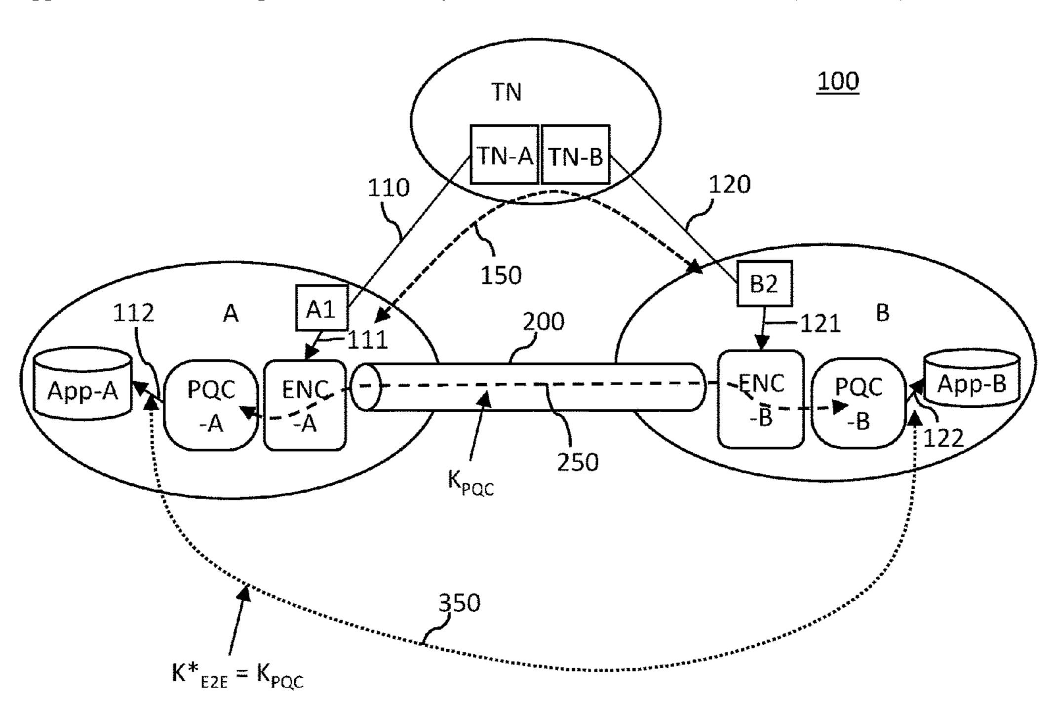
symmetrically encrypted channel between the first location and the second location using the quantum secured key. In the key agreement step, a first key agreement device at the first location and a second key agreement device at the second location together create an encryption key via the symmetrically encrypted channel.
