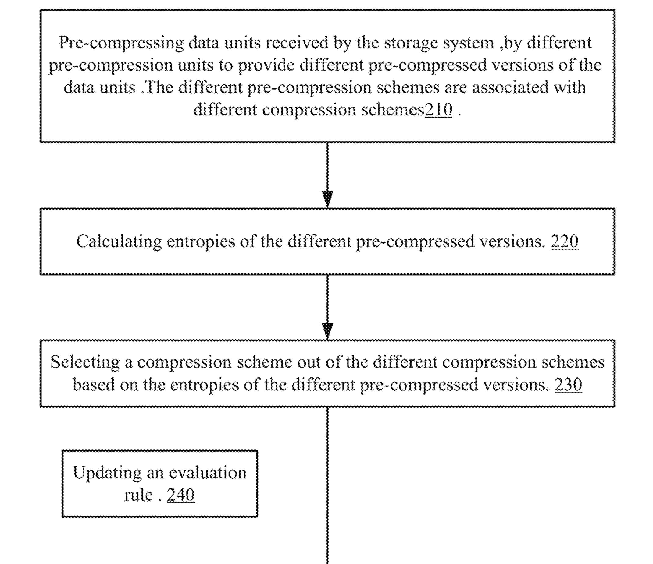
Compressing the data units by applying the selected compression scheme. <u>250</u>
