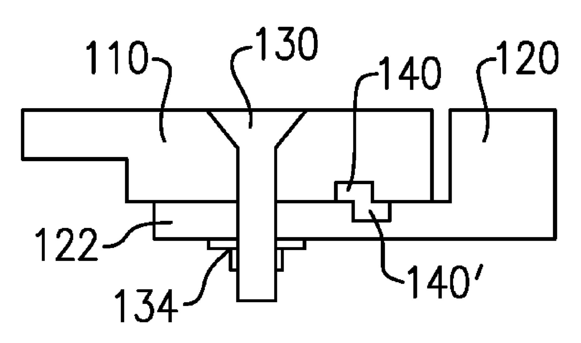
configured to maintain the relative positions of the first part and the second part. A channel is disposed on at least one of the radially inward facing surfaces and is positioned between the fastener and a circumferential edge of the first part. The channel is connected to at least one cooling air source.
