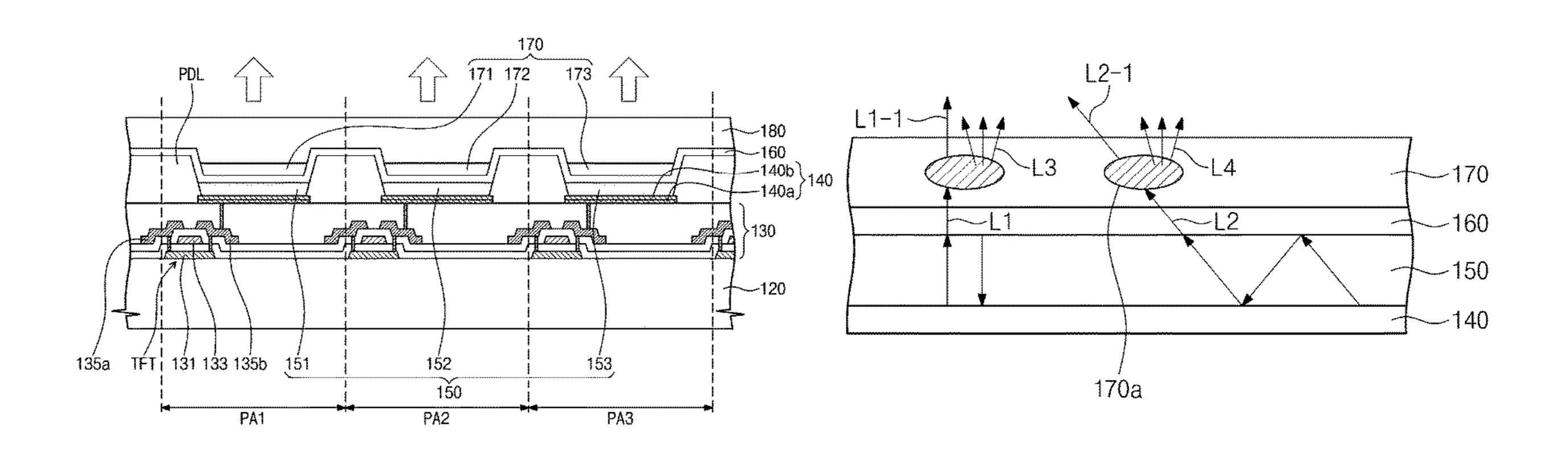
the sealing layer sealing the pixel electrode, the opposite electrode, the organic light emitting layer, and the light emitting layer.
