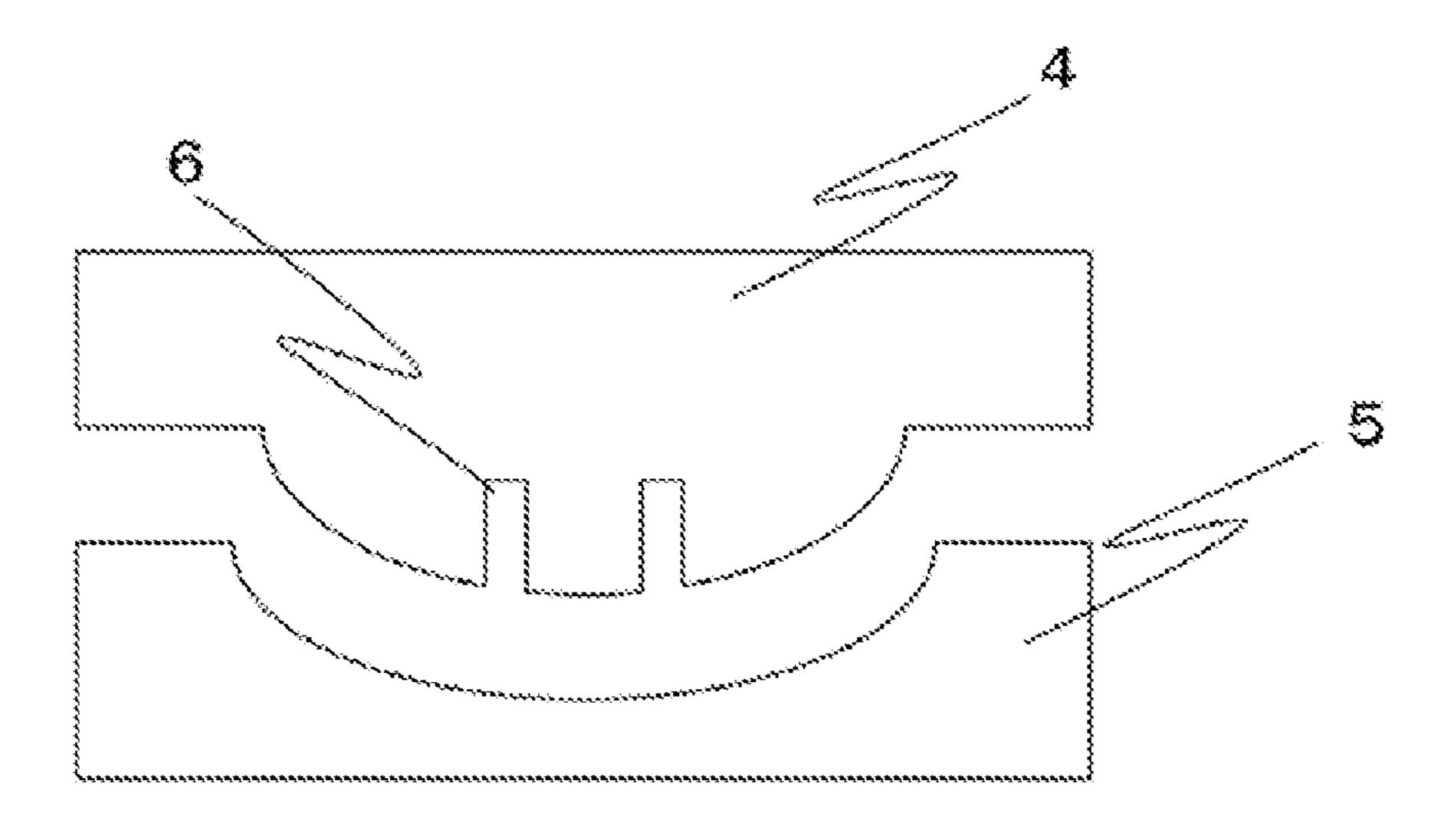
member having a recessed portion for forming a rib and a skin molding member free of such a recessed portion in a pressing device.
