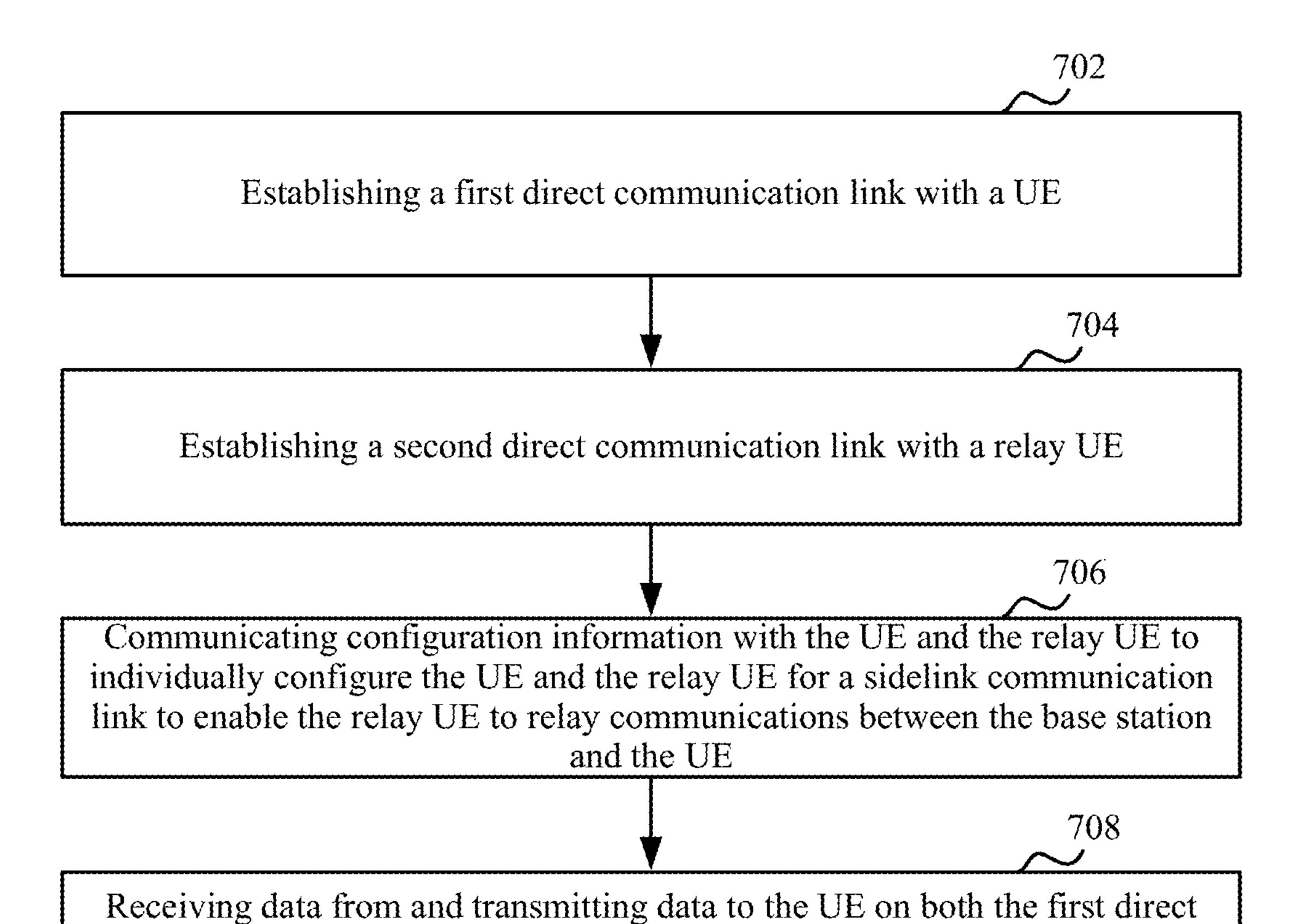
communication link and the second direct communication link in response to the sidelink communication link being established
