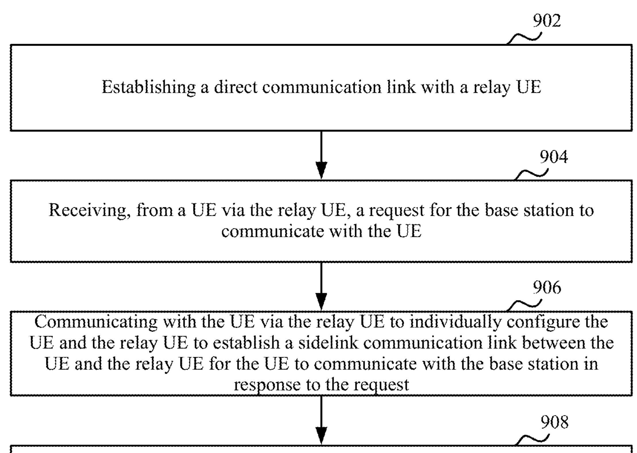
Receiving data from and transmitting data to the UE on the direct communication link, and via the sidelink communication link, in response to the sidelink communication link being established
