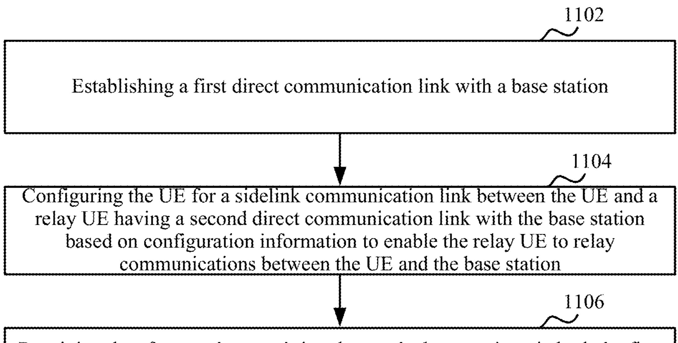
Receiving data from and transmitting data to the base station via both the first direct communication link and the sidelink communication link in response to the sidelink communication link being established
