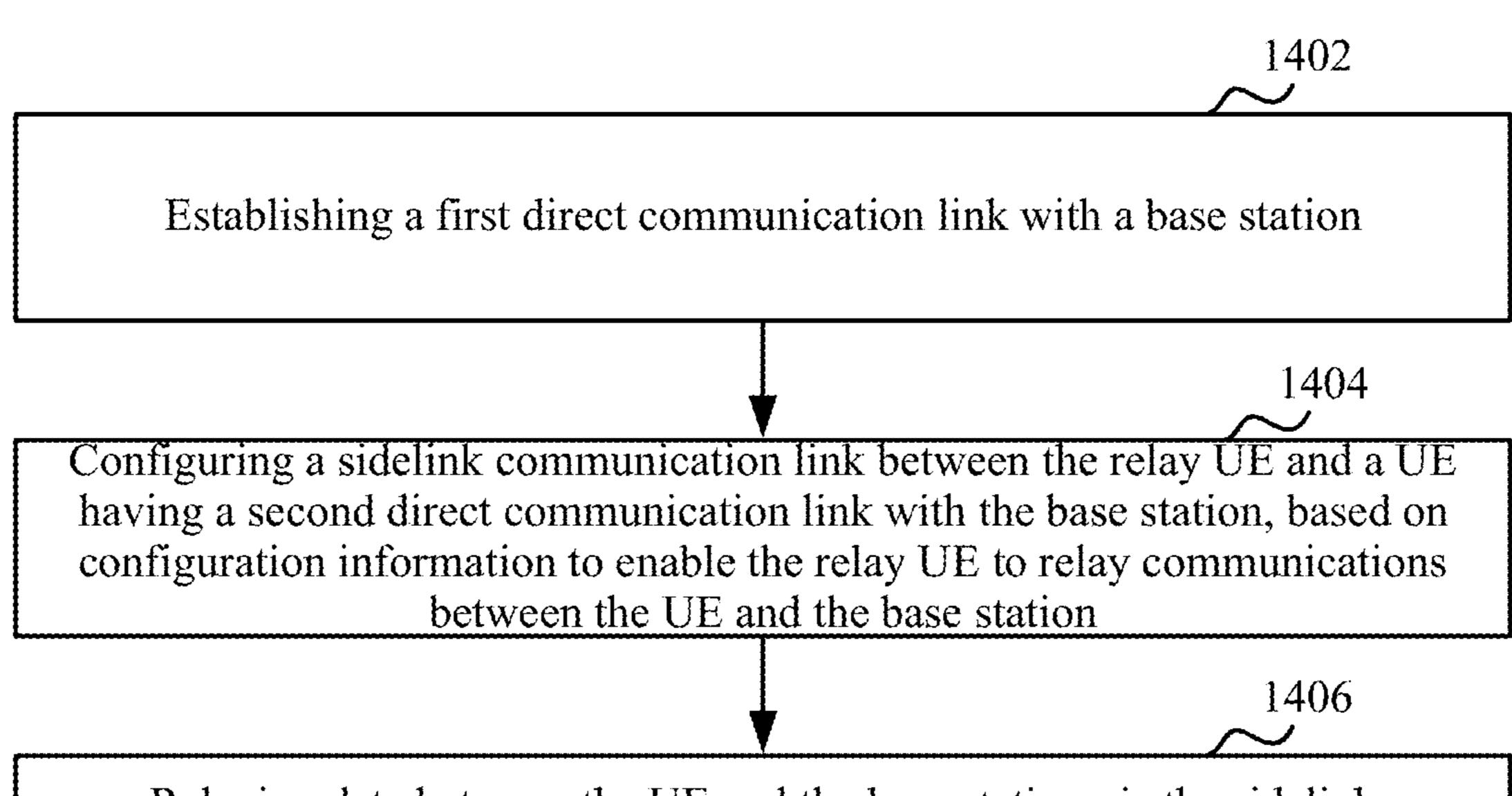
Relaying data between the UE and the base station via the sidelink communication link and the second direct communication link in response to the sidelink communication link being established
