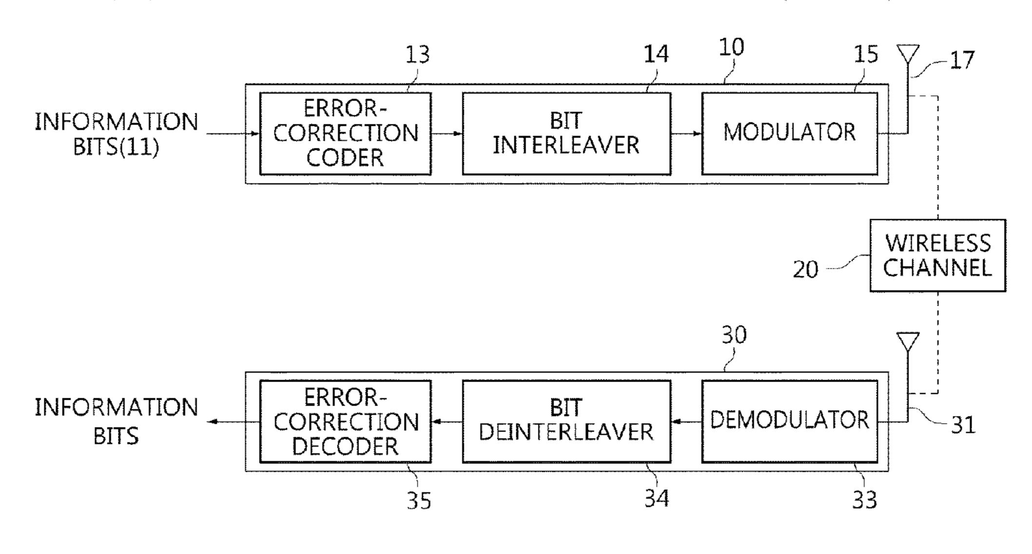
to a parallel factor of the LDPC codeword. The second memory provides the interleaved codeword to a modulator for quadrature phase shift keying (QPSK) modulation.
