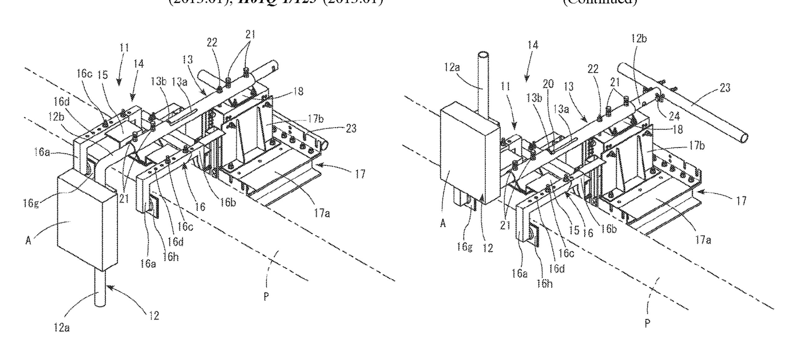
part is movable frontward/backward along a central axis thereof and is rotatable about the central axis. VSC part is made pullable to an inner wall side of the parapet by rotating HSC part about the central axis, and moving HSC part to the inner wall side of the parapet along the central axis.
