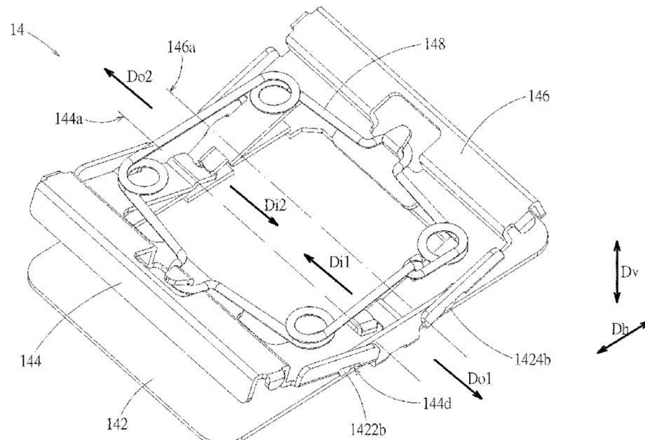
linkage portions push against each other in line contact, so that the two supports are mutually driven through the two linkage portions.
