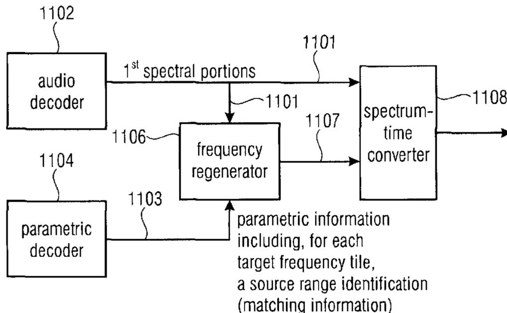
having a second spectral resolution being lower than the first spectral resolution; a frequency regenerator for regenerating every constructed second spectral portion having the first spectral resolution using a first spectral portion and spectral envelope information for the second spectral portion; and a spectrum time converter for converting the first decoded representation and the reconstructed second spectral portion into a time representation.
