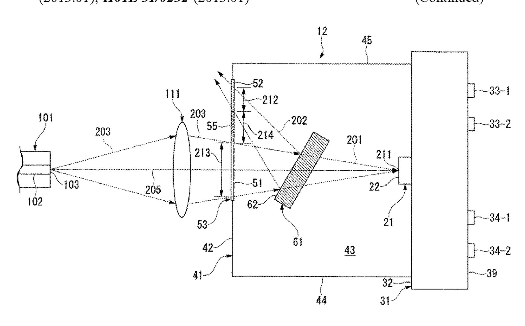
the housing between the window (51) and the photoreceptor (21) along the optical axis (205) of the optical signals (203), and that outputs, out of the optical signals (203) that enter thereto, the optical signals (201) toward the photoreceptor (21), and reflects the optical signals (202) toward a near side in a direction of travel of the optical signals (203).
