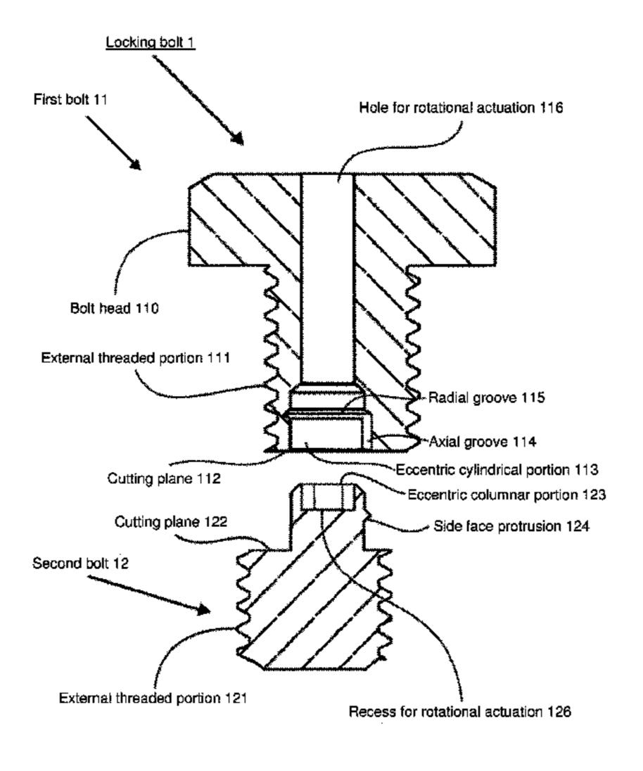
circumferential side face of eccentric columnar portion 123; first bolt 11 being such that eccentric cylindrical portion 113 that mates with eccentric columnar portion 123 is formed at cutting plane 112 in eccentric fashion with respect to a direction perpendicular to a central axis, axial groove 114 being formed in a direction parallel to the central axis and radial groove 115 being formed in a radial direction at the interior thereof; the entirety constituting locking bolt 1.
