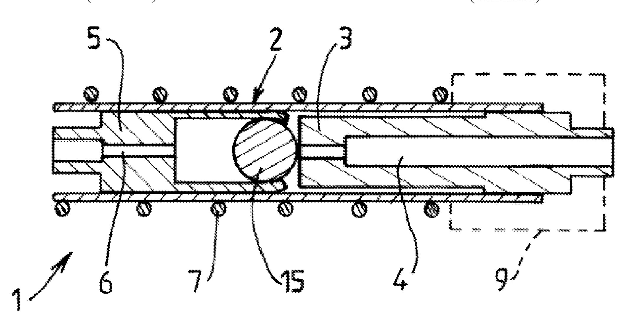
material having a different expansion coefficient from the piston or the nozzle, the valve comprising a heating member which, depending on the heating power delivered, makes it possible to separate the end of the nozzle and the piston by differential expansion, to allow the flow of fluid between the inlet and the outlet in an open position of the valve, characterized in that the terminal end of the piston comprises a ball that is crimped into the body of the piston.
