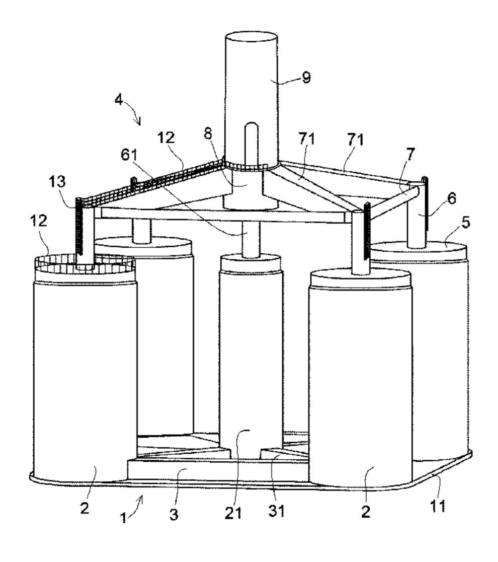
and the center of said lower slab; a metal superstructure supported on the concrete substructure and forming the base for connection with the wind turbine tower, said tower being coupled at the center thereof; and metal covers covering each of the cylinders, on which the metal superstructure is supported and to which vertical pillars are secured, linked together by beams, which join at the central pillar by an element whereon the base of the wind turbine tower is secured.
