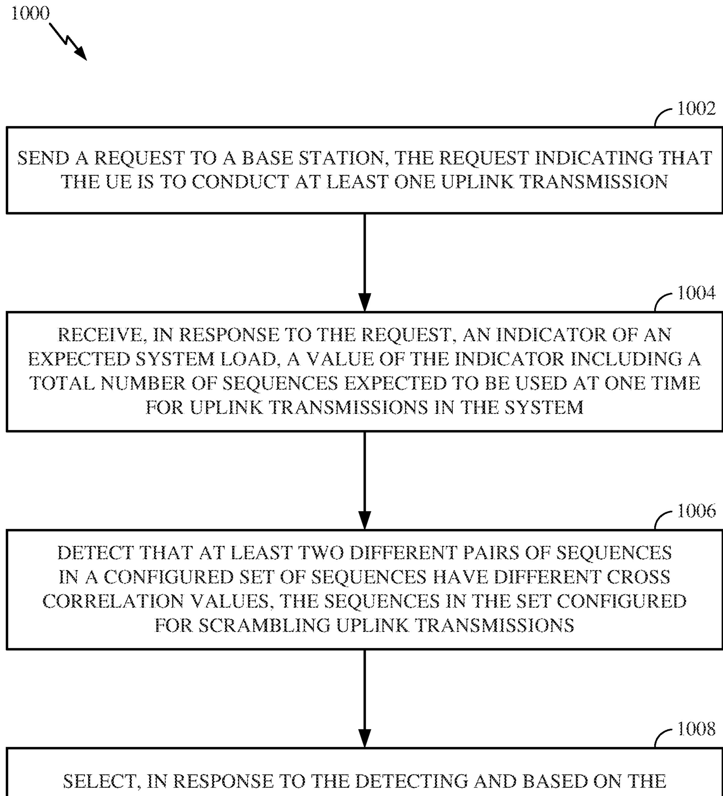
SELECT, IN RESPONSE TO THE DETECTING AND BASED ON THE INDICATOR, AT LEAST ONE SEQUENCE WITH AN IMPROVED CROSS CORRELATION WITH AT LEAST ONE OTHER SEQUENCE, THE AT LEAST ONE SEQUENCE AND THE AT LEAST ONE OTHER SEQUENCE TO BE USED FOR SCRAMBLING UPLINK TRANSMISSIONS WITHIN THE SYSTEM
