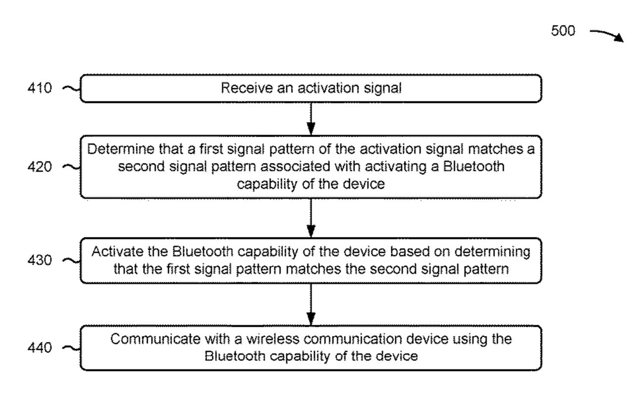
Determine signal pattern associated with activating a Bluetooth capability of a user device
