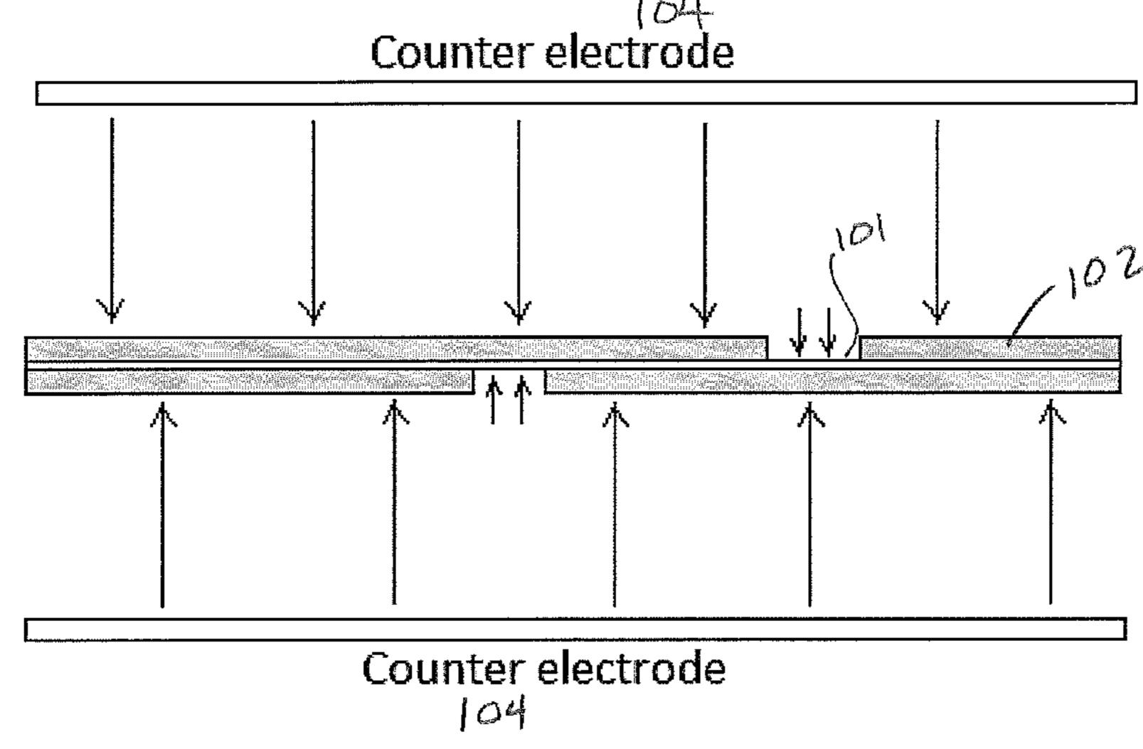
Double side coated anode substrate
