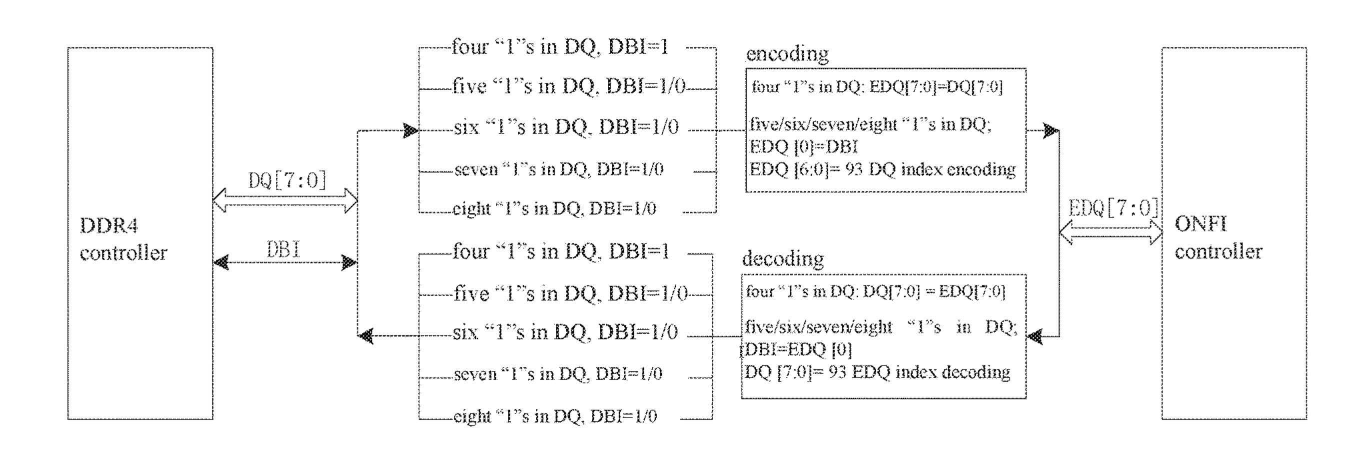
to the values of the N-bit DQ and the 1-bit DBI, and sending the N-bit EDQ to the NAND flash memory controller; and receiving, by the NAND flash memory controller (102), the N-bit EDQ and writing the N-bit EDQ into the NAND flash memory (202).
