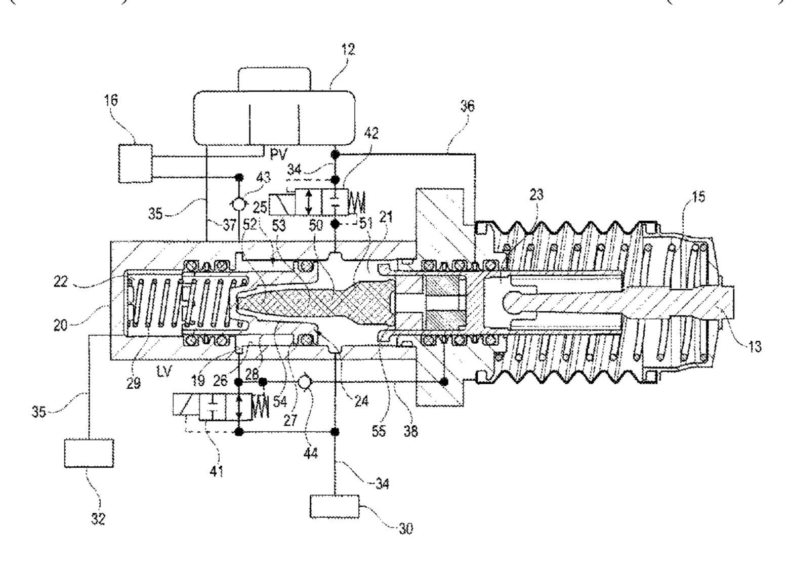
locking chamber and an elastic pedal feel element arranged in the first master chamber to be in contact with the first master piston and the second master piston for generating a pedal force when the brake pedal is operated while the second master piston is locked in the normal operating mode.
