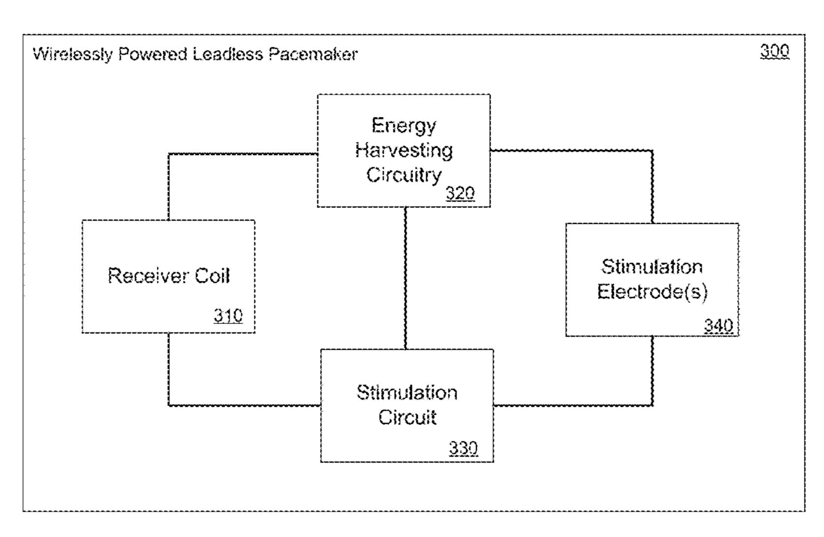
using the first wireless power signal generator, and transmit the power transfer signal using the wireless power transmitter, wherein the wirelessly powered, leadless pacemaker receives the power transfer signal using the first wireless power receiver, and when receiving the power transfer signal, the energy harvesting circuitry stores power received via the wireless power receiver in at least one capacitor.
