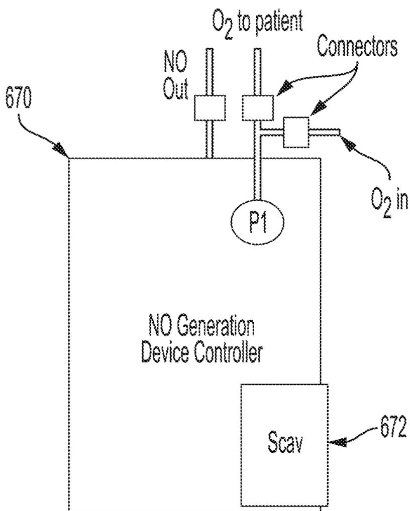
Device design that measures O<sub>2</sub> pressure to detect respirations and synchronize gas delivery
