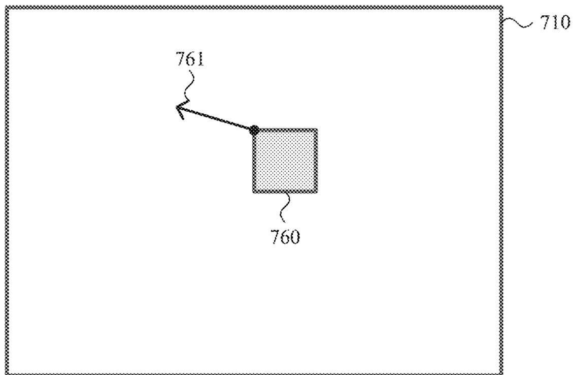
default BV predictor of (0, 0) for BV (761) for current block (760) of current frame (710)
