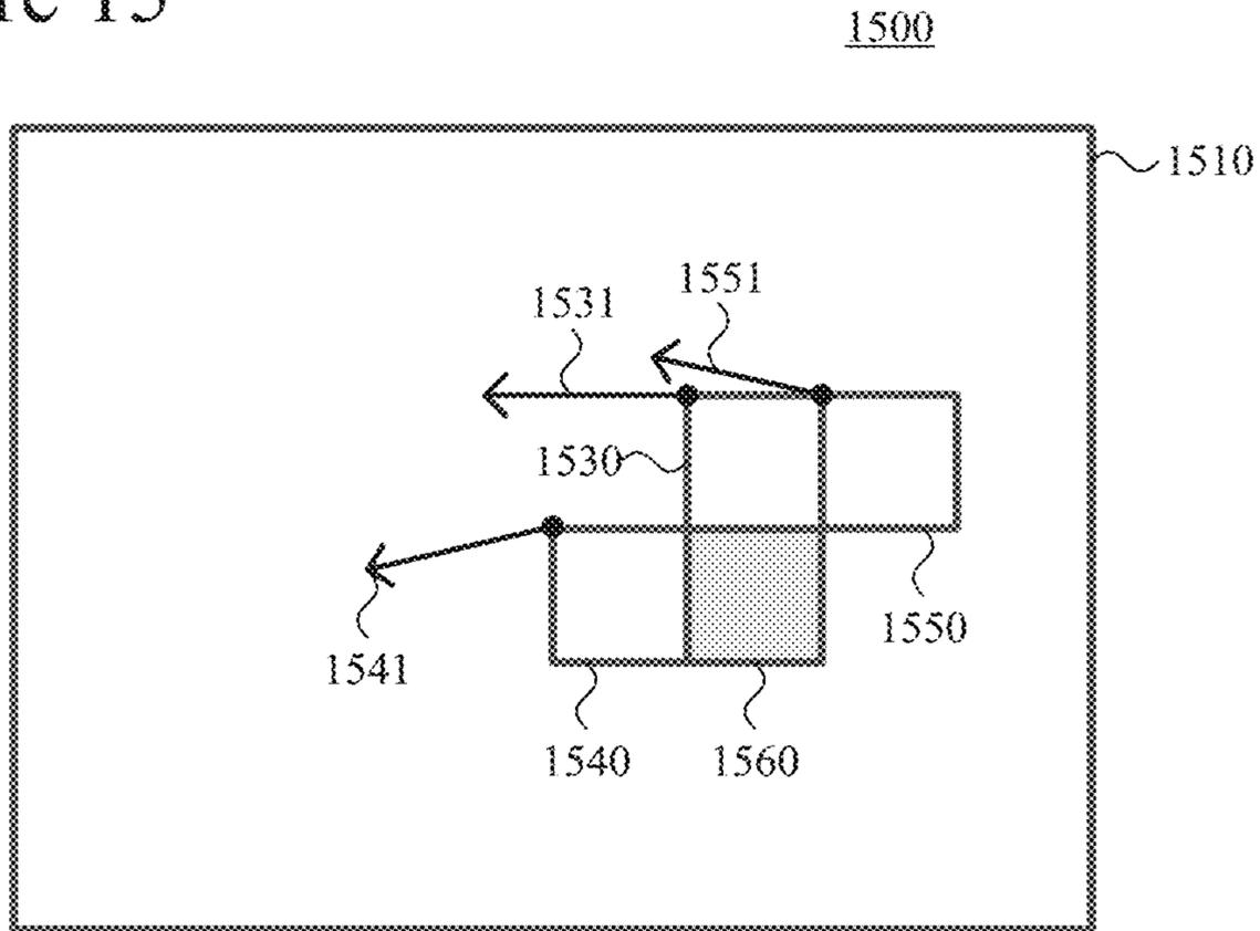
BV predictor candidates from BV values (1531, 1541, 1551) of three neighboring intra-BC-predicted blocks according to merge mode for BV for current block (1560)
