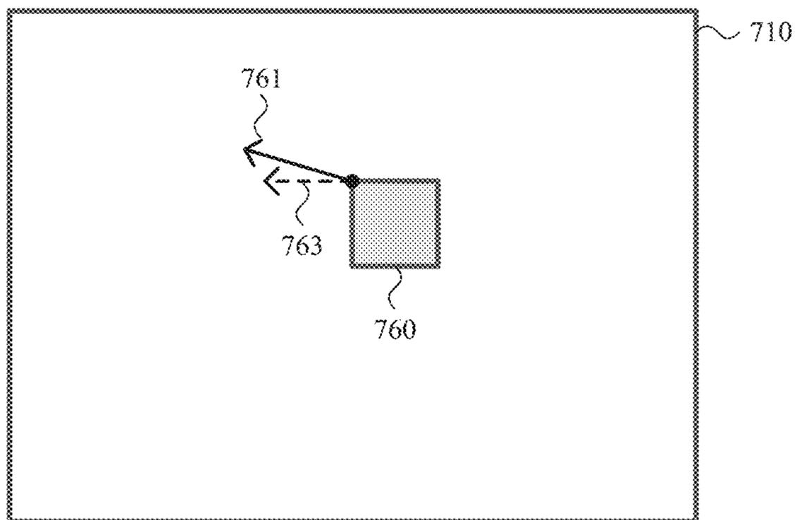
default BV predictor (763) with non-zero horizontal component for BV (761) for current block (760) of current frame (710)
