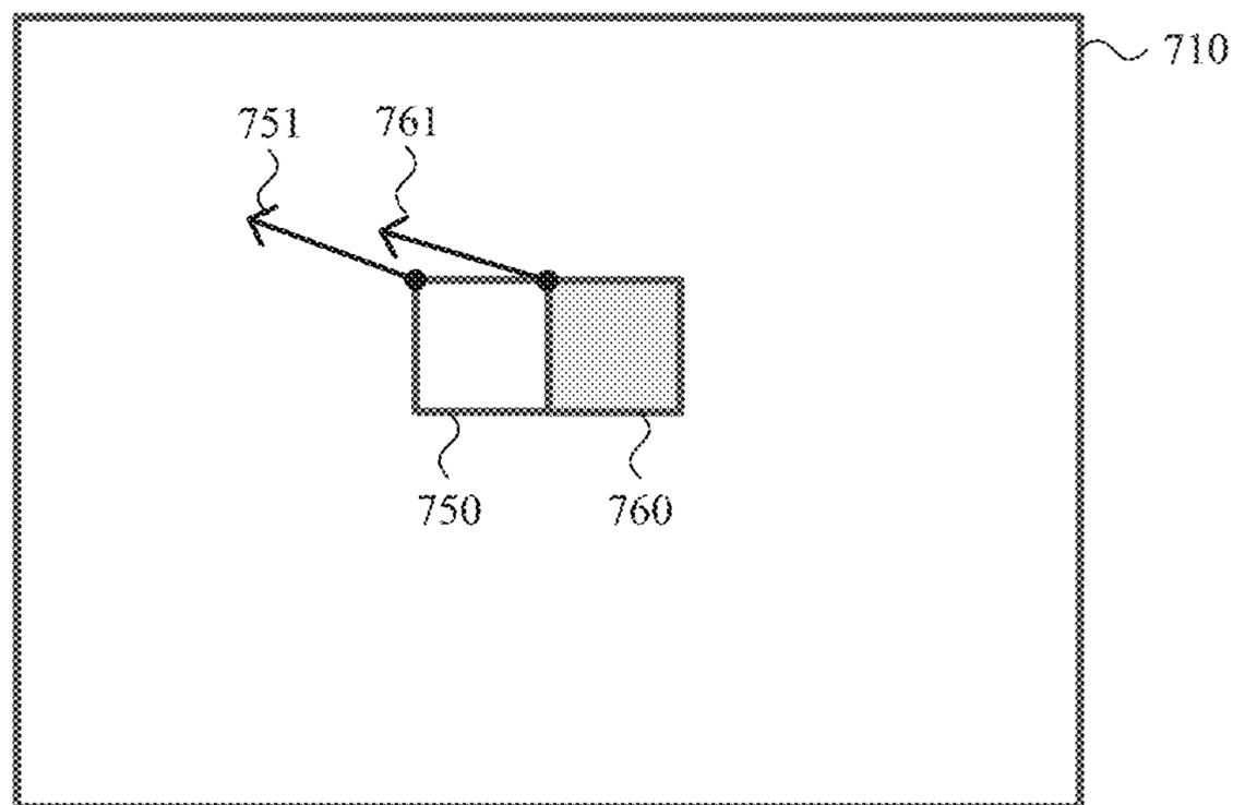
BV (751) of previous intra BC predicted block (750) used as BV predictor for BV (761) for current block (760) of current frame (710)
