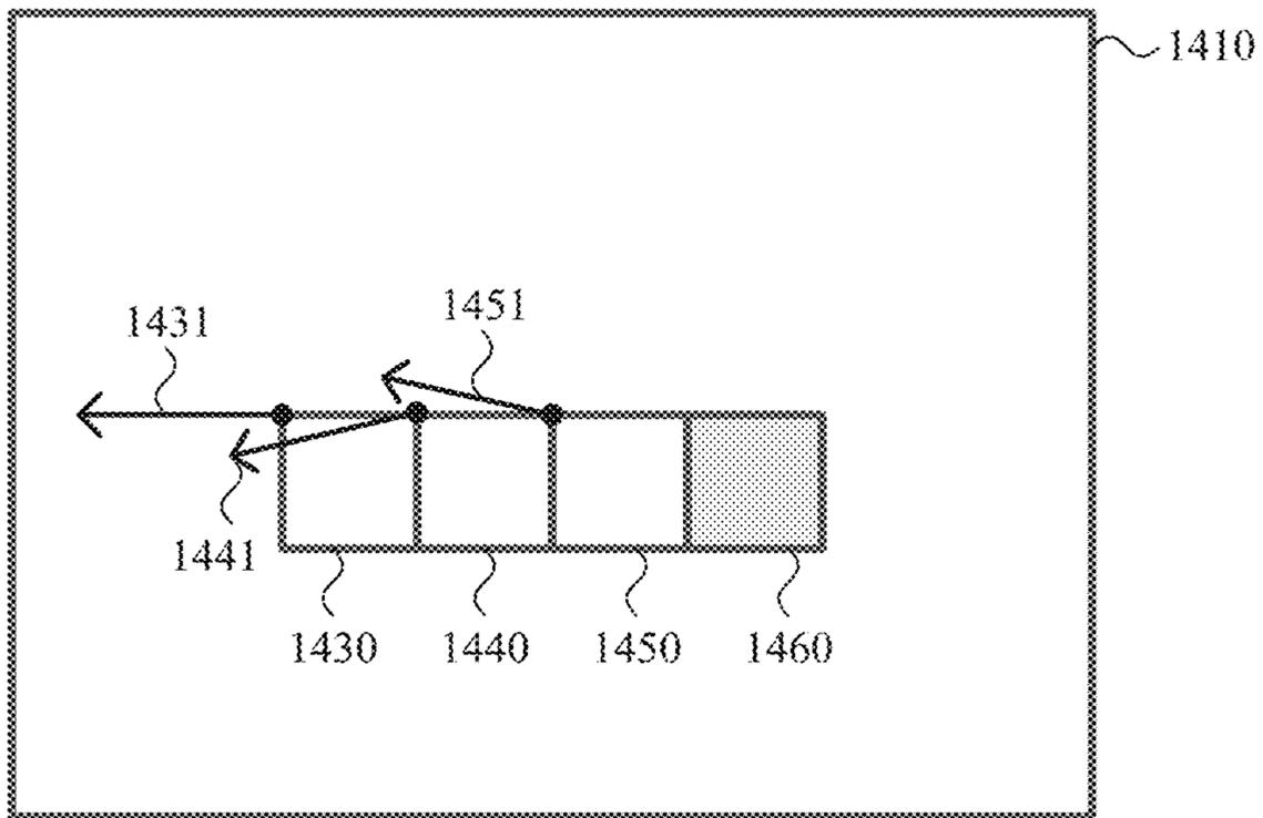
BV predictor candidates from BV values (1431, 1441, 1451) of three previous intra-BC-predicted blocks according to merge mode for BV for current block (1460)
