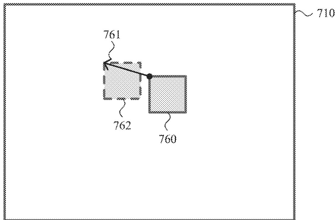
BV (761) for current block (760) of current frame (710), indicating a displacement to a matching block (762) in the current frame (710)
