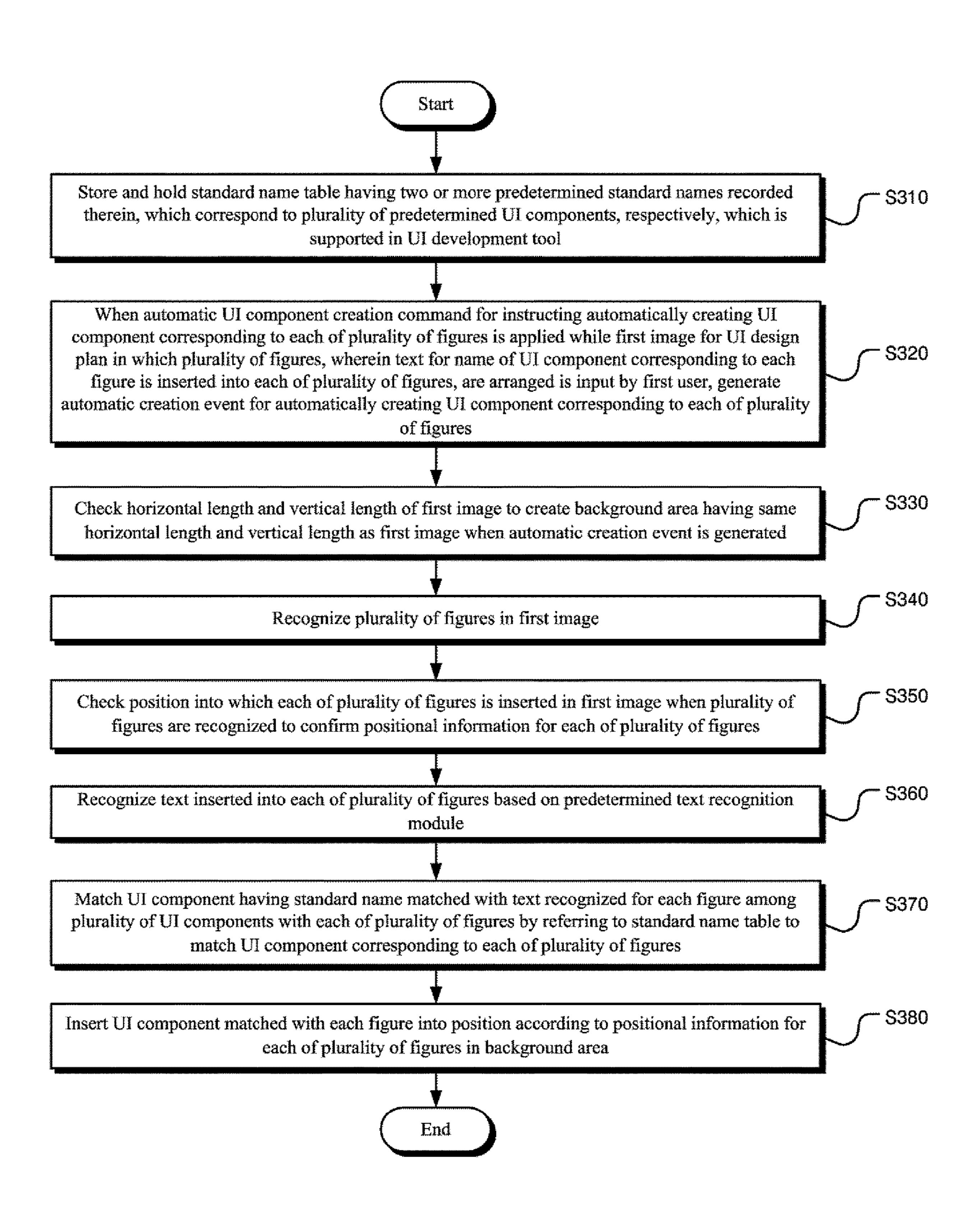
ELECTRONIC TERMINAL APPARATUS EQUIPPED WITH THE UI DEVELOPMENT TOOL, WHICH IS ABLE TO PROVIDE AN AUTOMATIC UI COMPONENTS CREATION FUNCTION THROUGH IMAGE ANALYSIS OF A UI DESIGN PLAN, AND THE **OPERATING METHOD THEREOF**
