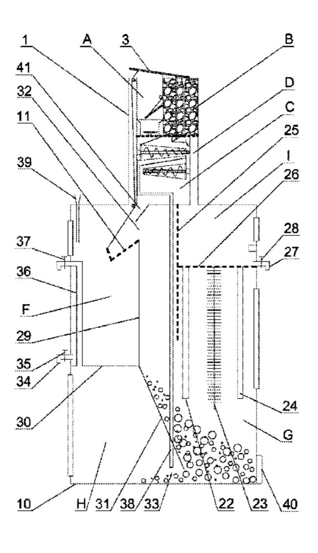
solid residue particles. The solid residue particles degrade and adsorb pollutants in the water after being activated by an acidic solution. Meanwhile, accumulated water-absorbing solid residue particles help to degrade the pollutants in the water through the electrolysis device. A separation area is configured to separate oil and discharge the oil separately.
