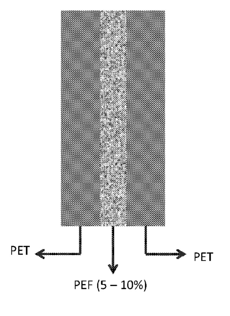
layers, has been found to achieve a significantly higher barrier against gas permeation relative to conventional monolayer PET container of the same size and shape. Associated preforms, methods, and compositions are disclosed.
