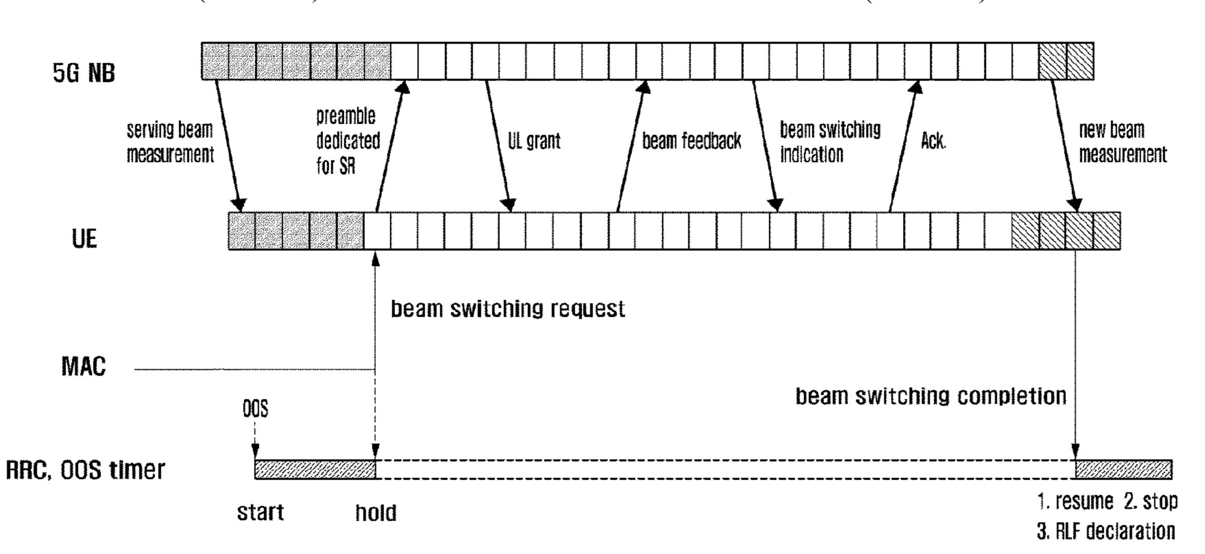
synchronization (OOS) with respect to a plurality of reception beams; starting a timer to determine a radio link failure when the indication of OOS is identified; and holding the timer when at least one of the plurality of reception beams is requested to be changed.
