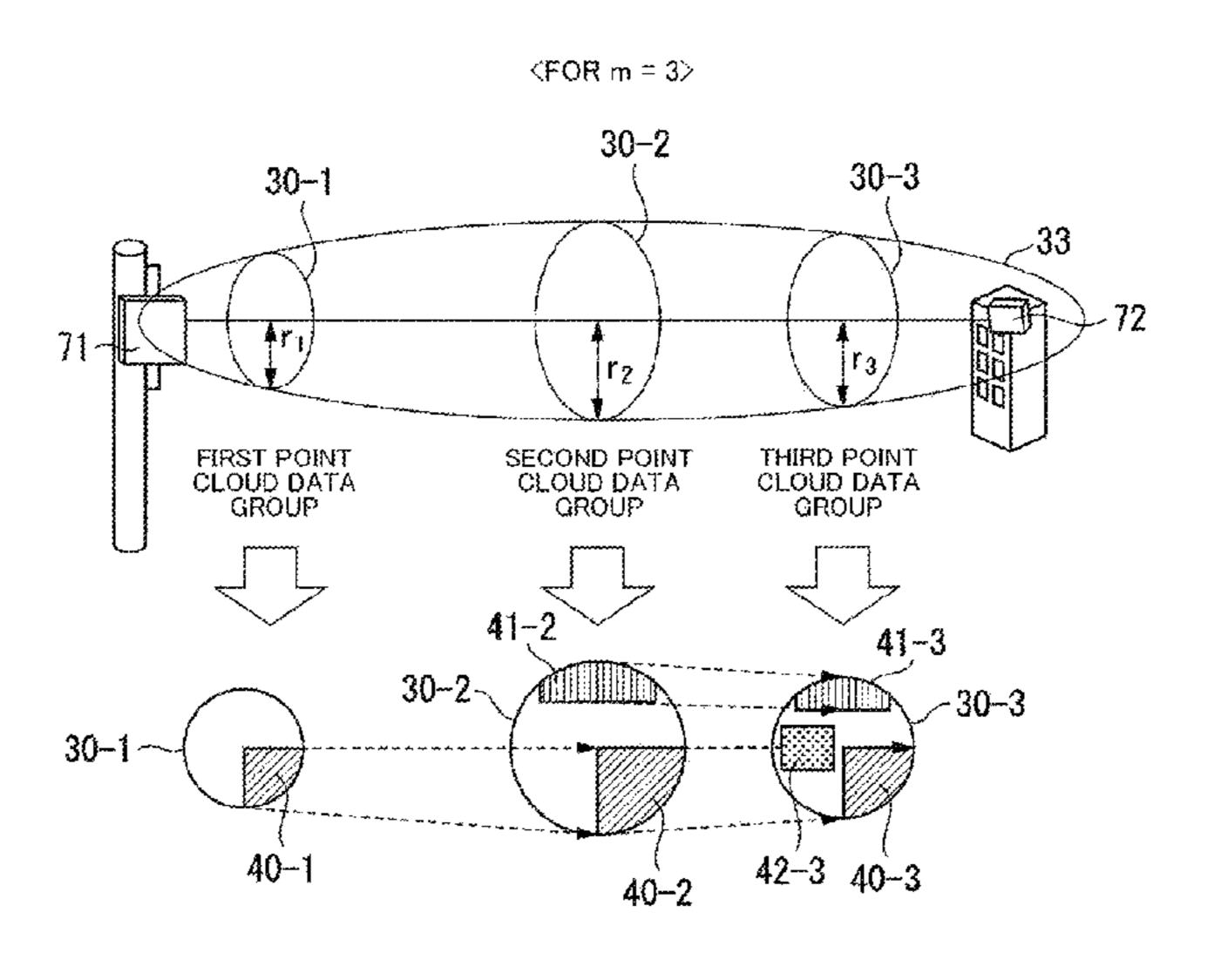
line-of-sight regions to an area of a region constructed by the first Fresnel zone is calculated. A received power is estimated based on the calculated ratio between the areas. Whether or not there is a line of sight between the base station device and the terminal station device is determined based on the received power.
