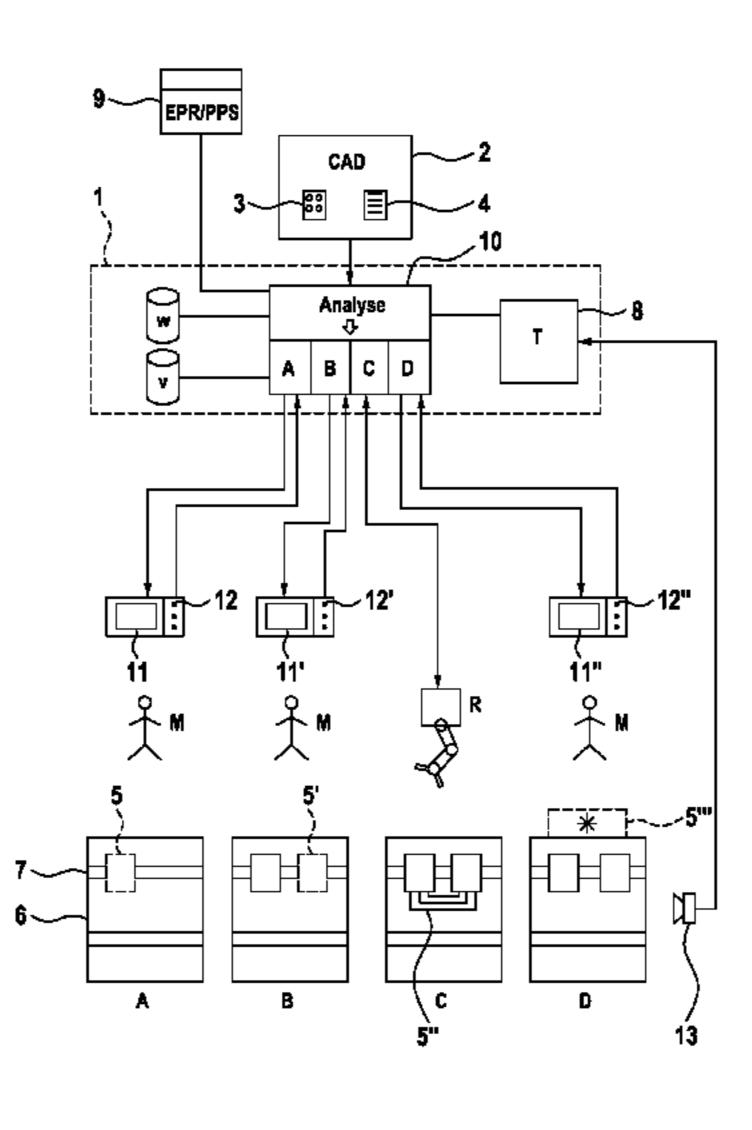
sequence. The system and method further includes at least one input unit (12-12') for acknowledgement of the completed assembly step (A; B; D) by the fitter (M).
