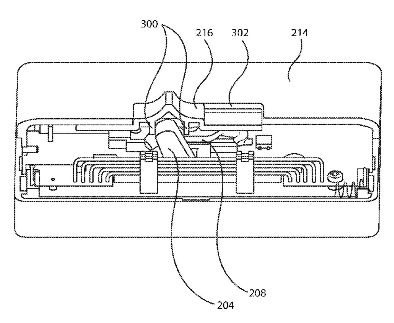
toggle member to place the toggle light switch member into the on position.
