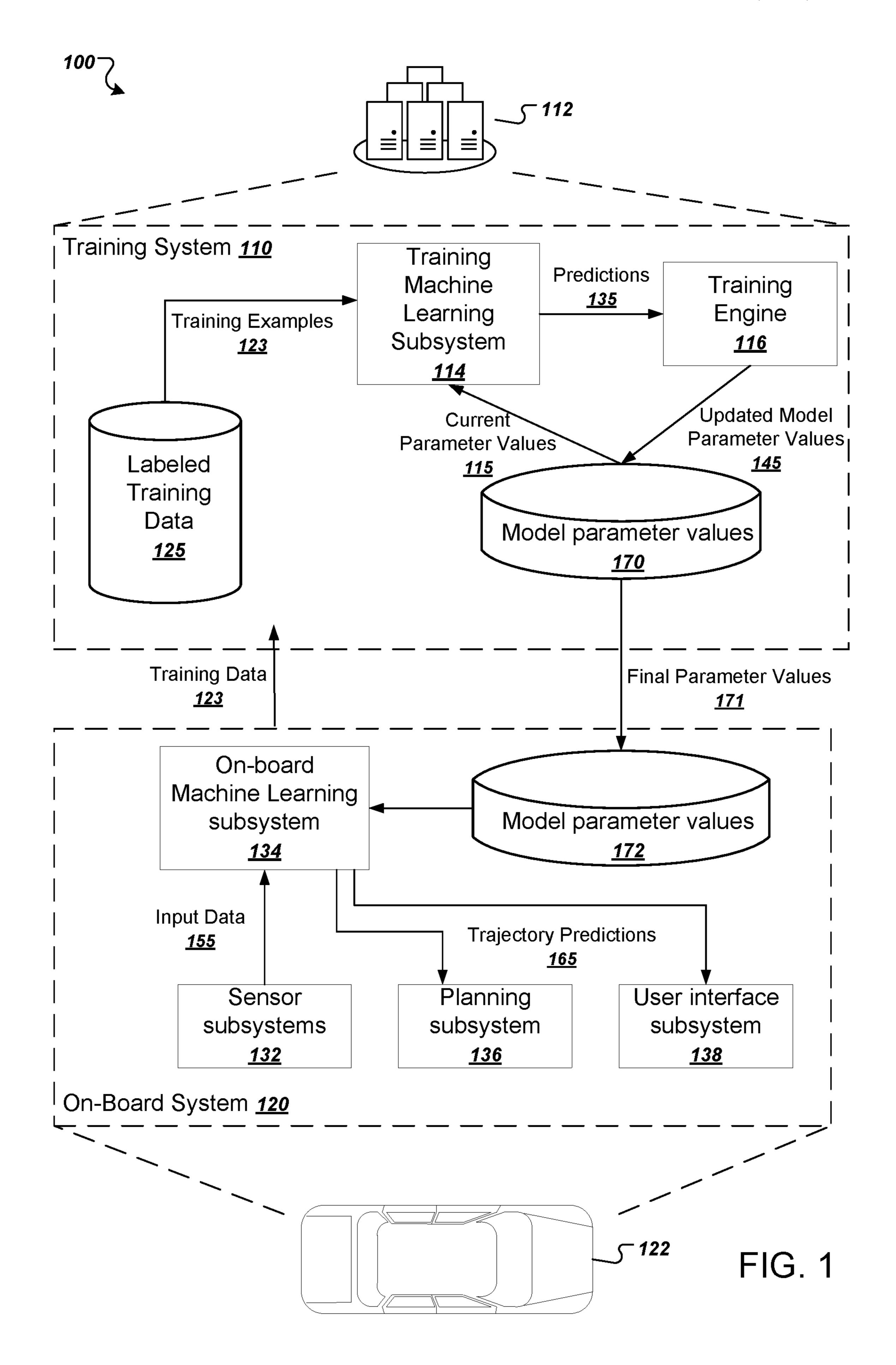
Obtain a training input for training a machine learning model to perform trajectory prediction, the training input including (i) data characterizing an agent in an environment as of a first time and (ii) data characterizing a candidate trajectory of the agent in the environment for a first time period that is after the first time
