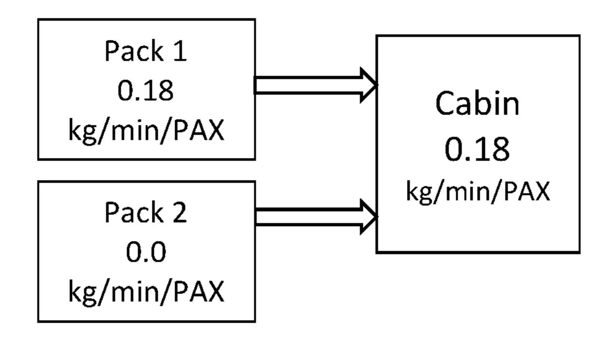
Packs sized for failure flow
