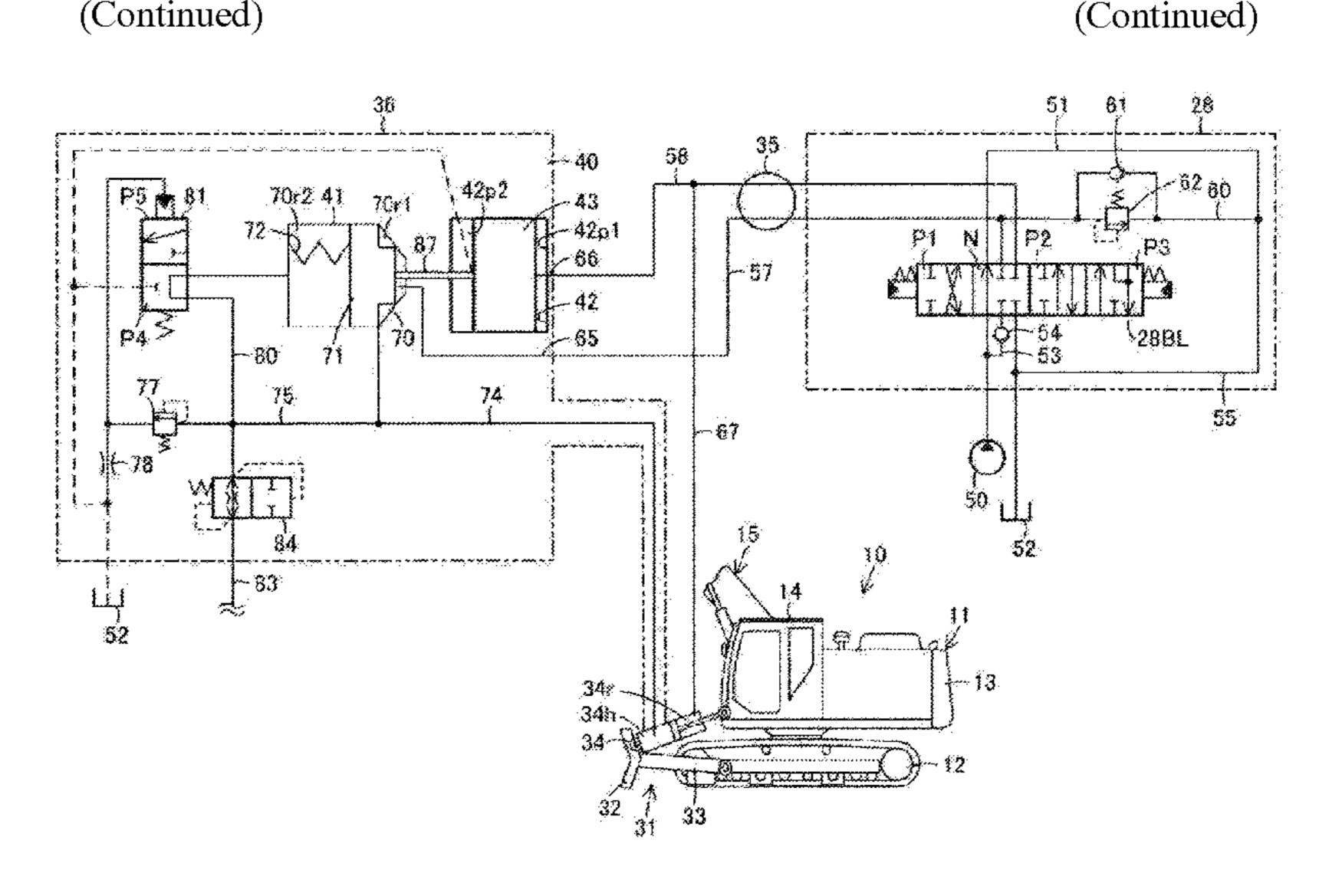
is connected to the poppet 71 of the non-return valve 41, so that the power piston 43 can be operated by the difference between the urging force of the poppet 71 by a spring 72 of the non-return valve 41 and a rod chamber pressure of the blade cylinder 34.
