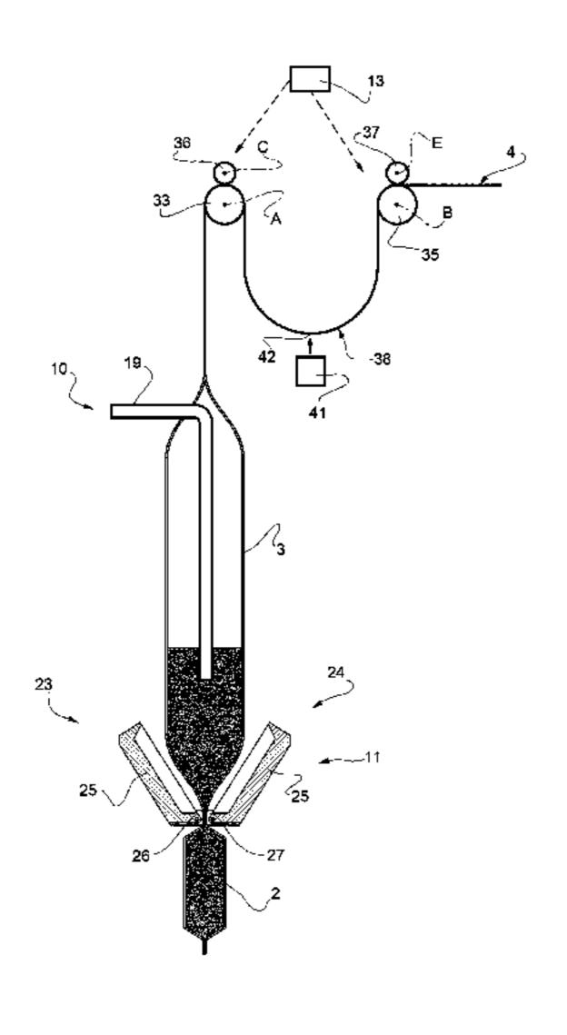
prises a main drive roller rotatable around a main rotation axis and a main drive motor configured to actuate rotation of the main drive roller around the main rotation axis. The control unit is configured to control the main drive motor such that angular speed and/or angular acceleration of the main drive roller is cyclically varied to control the tension of the tube.
