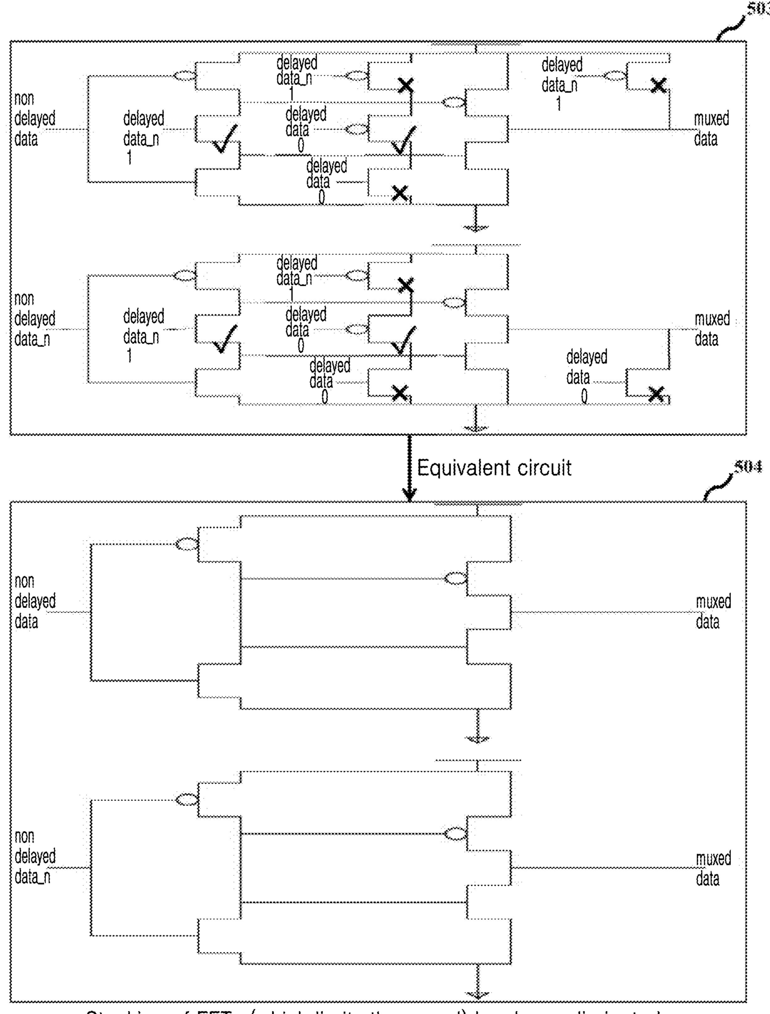
Stacking of FETs (which limits the speed) has been eliminated
