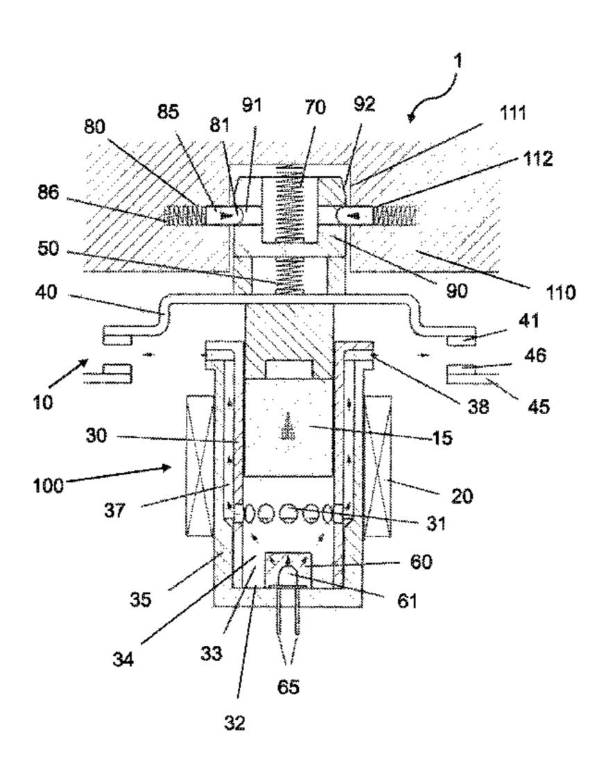
The switching device further includes an electromagnetic switching drive with a coil for generating a magnetic field and a magnet anchor, a guide sleeve to guide the movement of the magnet anchor in the magnetic field of the coil, a pyrotechnic propellant charge located in the cavity, and a supporting device for supporting the guide sleeve. The magnet anchor is arranged within the guide sleeve such that a cavity is formed below the magnet anchor.
