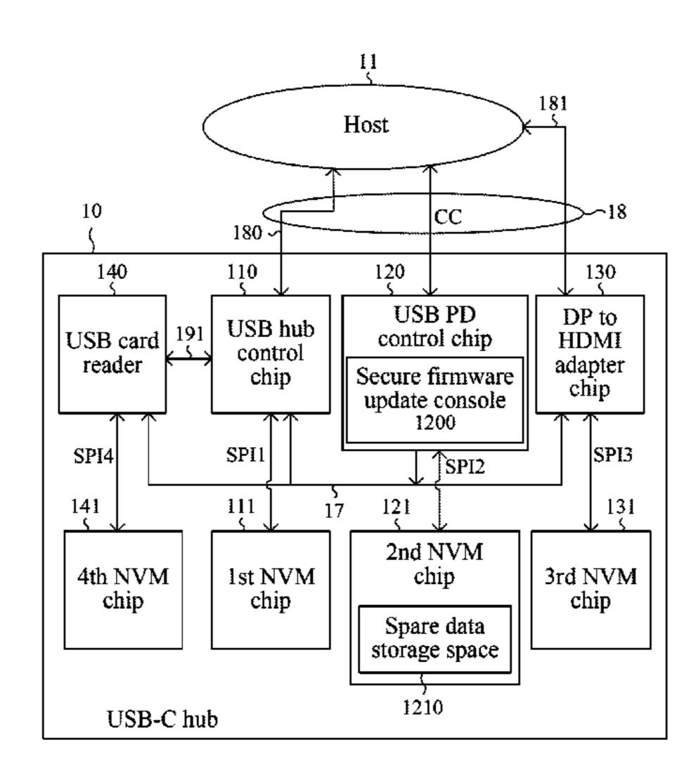
chip to overwrite the second firmware code after passing a verification procedure on the firmware code update data.
