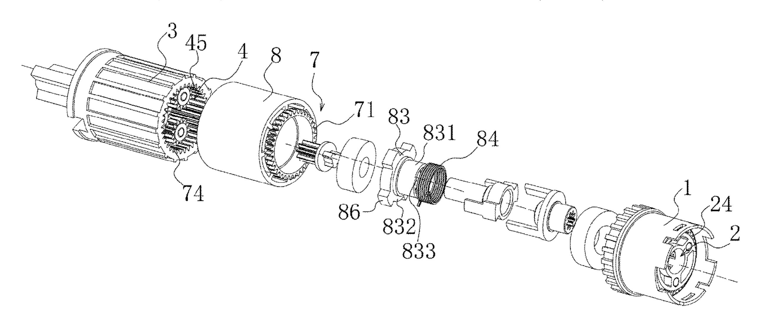
driving member is in transmission connection with the brake driven member, and a braking assembly connected to the brake driving member and the brake driven member is provided on the inner side of the brake outer sleeve in the circumferential direction.
