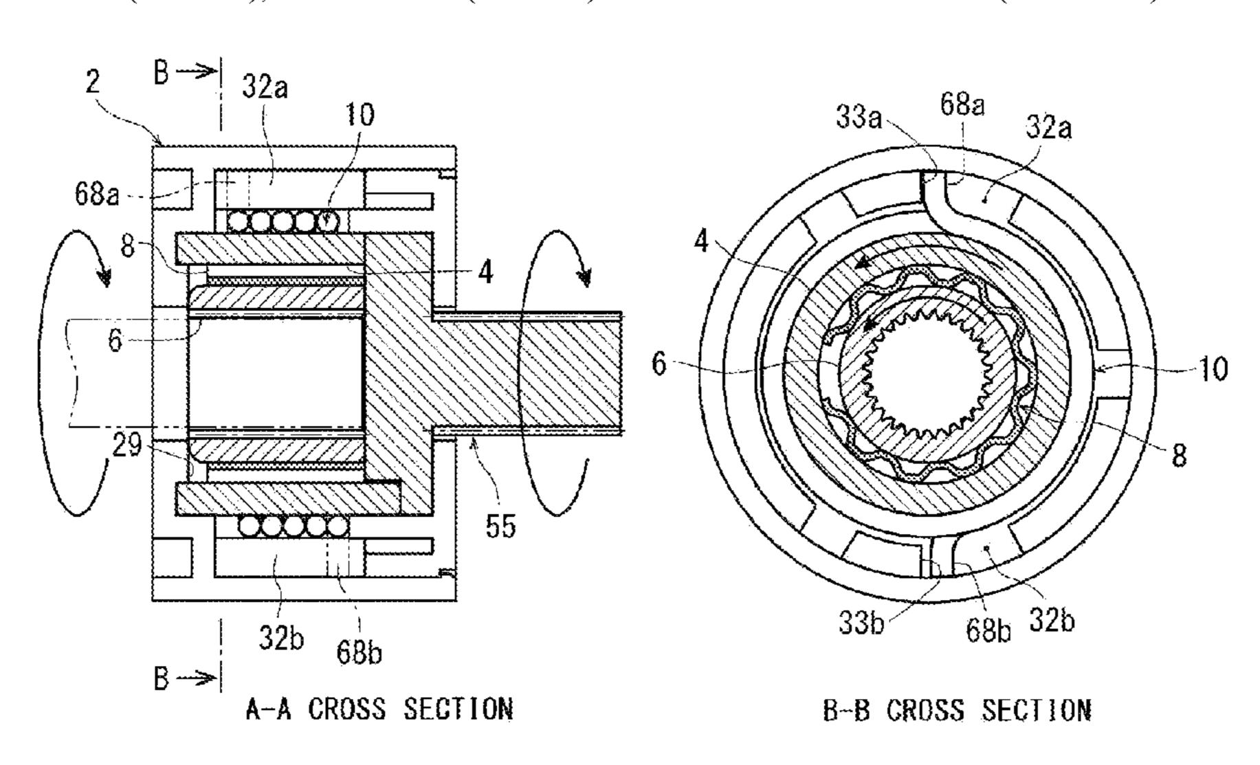
from the input-side device becomes excessive, slippage occurs on the thin-plate elastic piece, whereby the outer and inner race members are disconnected.
