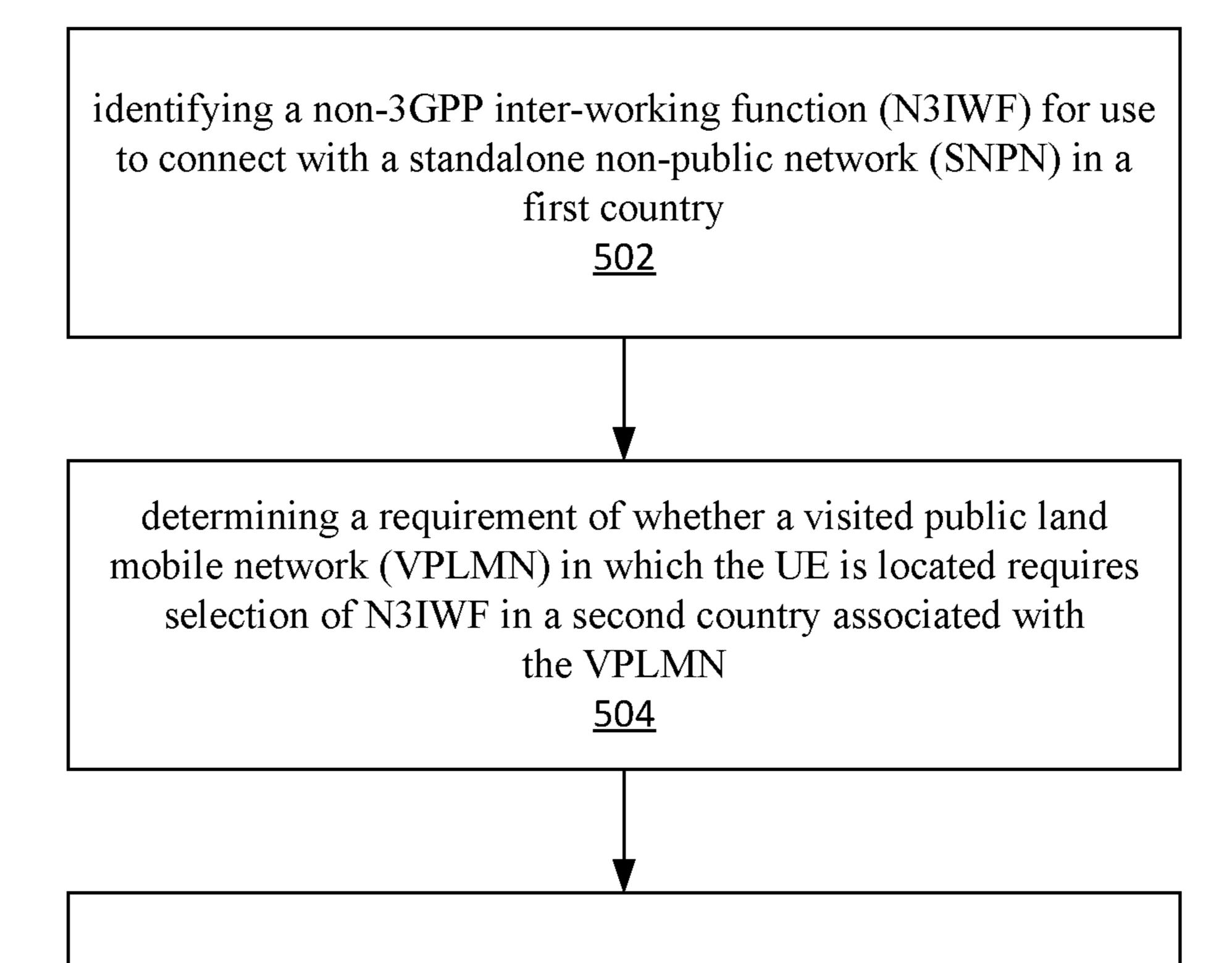
determining whether to connect to the SNPN with the identified N3IWF based on the determined requirement 506
