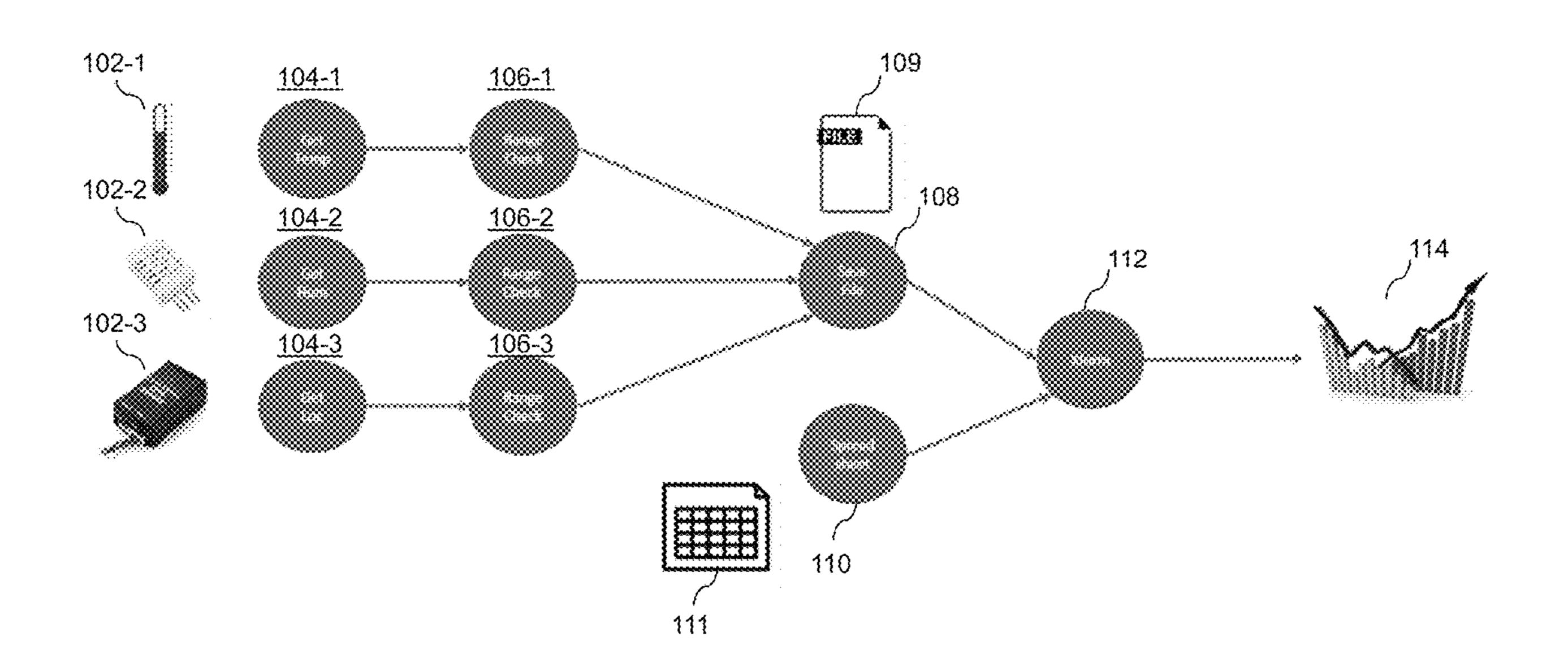
data obtained by the given gateway node from the corresponding one or more sensors. A data flow valuation operation is performed at the given gateway node based on the executed data flow to generate a data flow valuation result.
