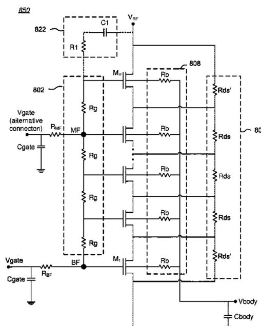
ders for the FET gate resistors, drain-source resistors, body charge control resistors, and one or more AC coupling modules.
