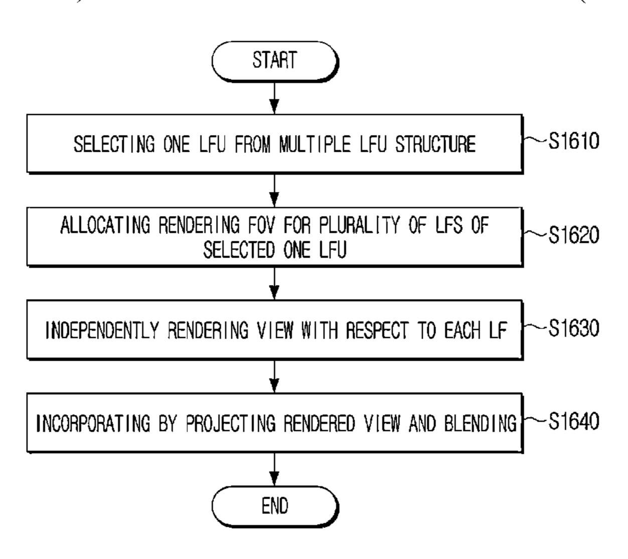
a plurality of view images based on a plurality of light fields comprising the selected LFU and the allocated FOV, and generate the 360-degree image by incorporating the generated plurality of view images.
