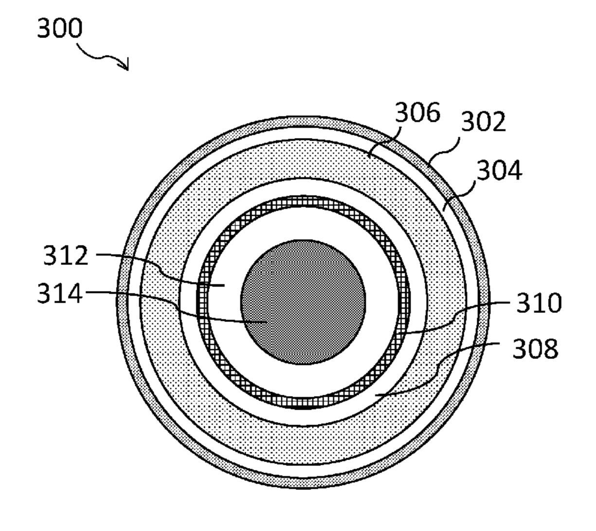
guide cladding disposed around the second intermediate cladding, and outer cladding disposed around the waveguide cladding, and an outer coating around the outer cladding. An optical fiber may be formed using a rod-in-tube process.
